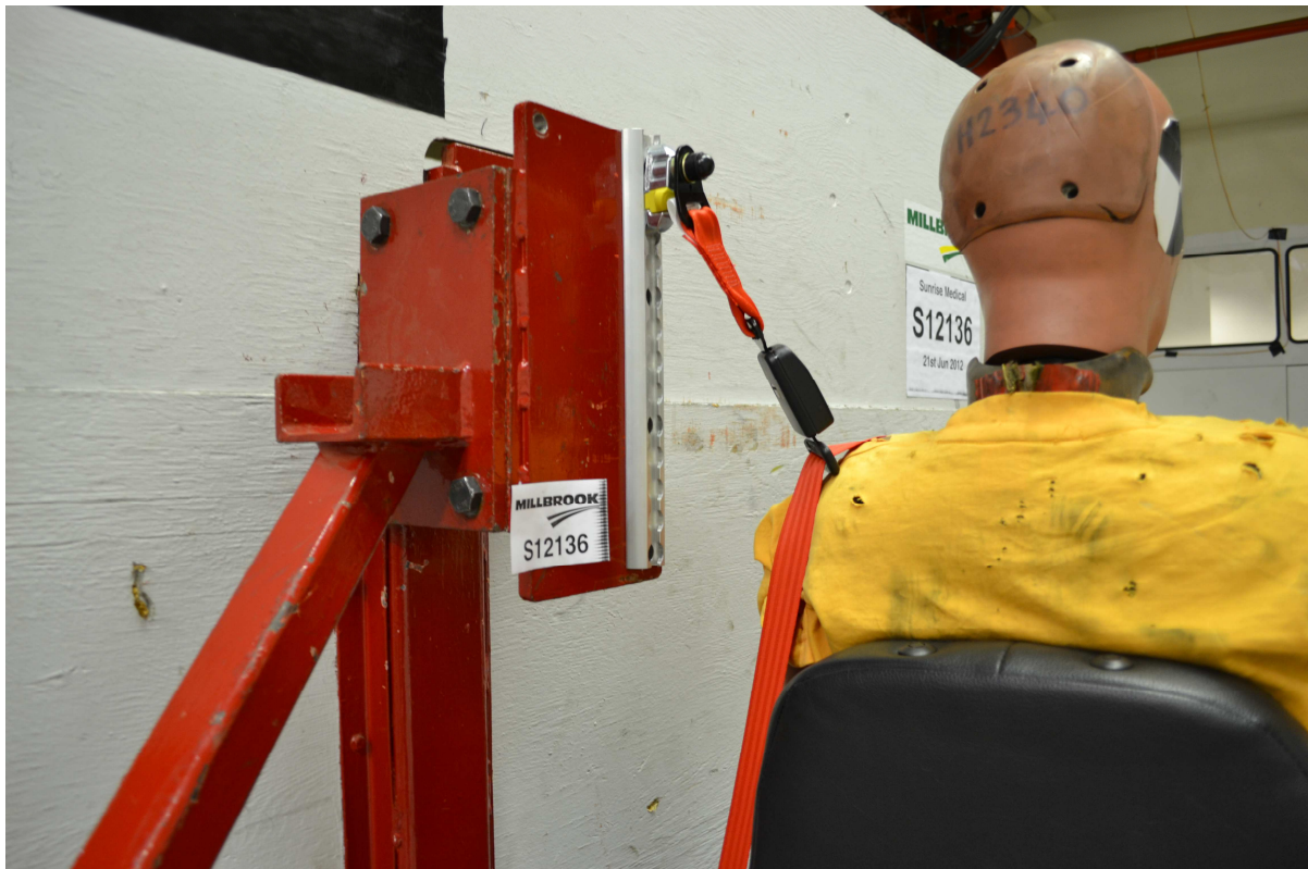
Occupant restraint anchorage point, pre-test
