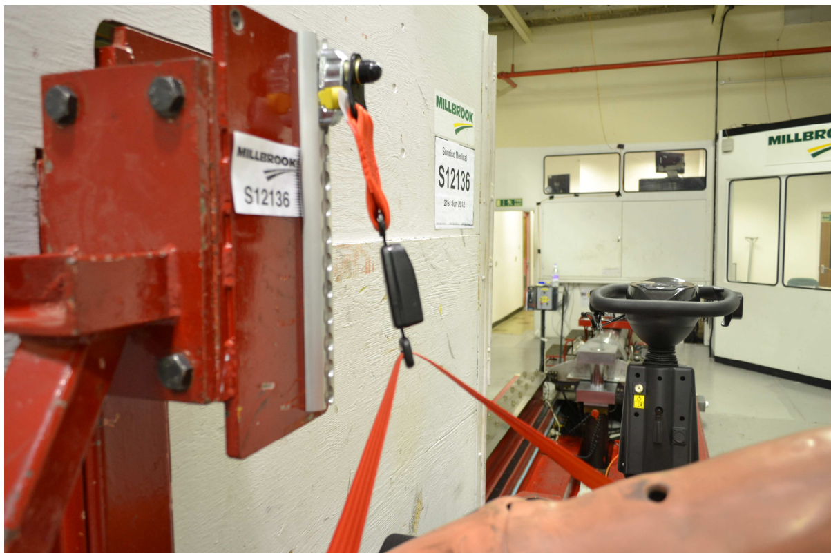
Occupant restraint anchorage point, post-test
