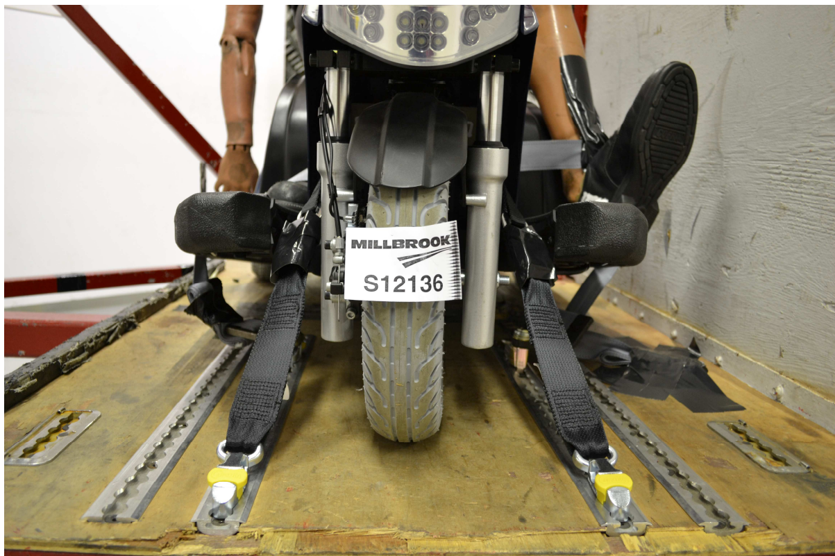
Front wheelchair restraints, post-test
