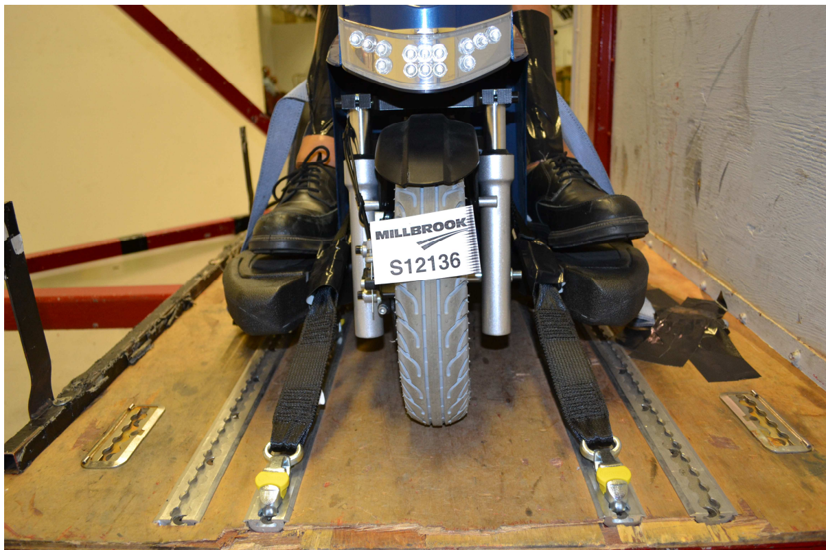
Front wheelchair restraints, pre-test
