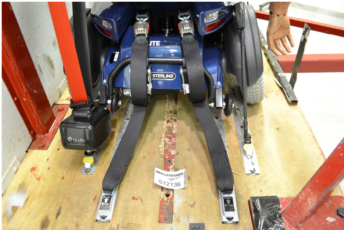
Rear wheelchair restraints, post-test
