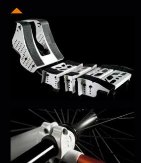
A NEW rear axle with forged parts combines high stability with low weight.
