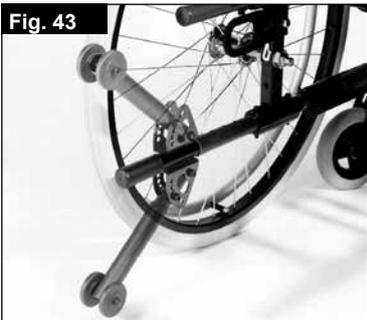
By pushing on the Second exposed release button, the safety wheels can be set upwards or removed. There must always be a gap of between 3 cm and 5 cm between the tube and the ground. You must swing the safety wheels upwards when going up and down large obstacles (such as a kerb) to prevent them from touching the ground. Then rotate the safety wheels back down to the normal position (Fig. 43).
