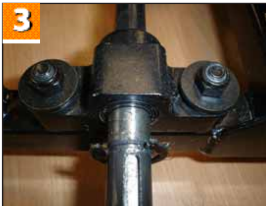
3. Location of the other 2 transaxle mounting bolts.
