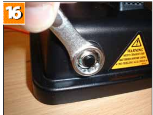
16. Using a 14mm ring spanner undo the power cut out nut.
