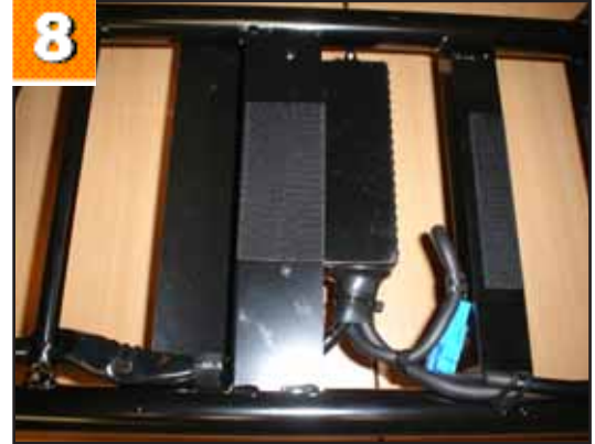
8. Shows the controller and main wiring looms.
