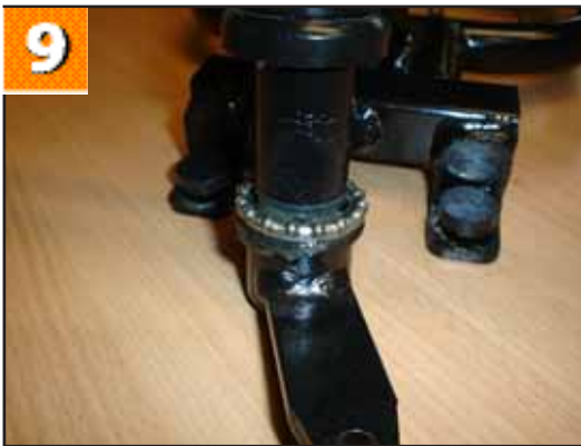
9. Lower the steering head bracket out of the frame. NOTE: This is only possible when the Front Frame Bump Stops have been removed. (See Chapter 16).
