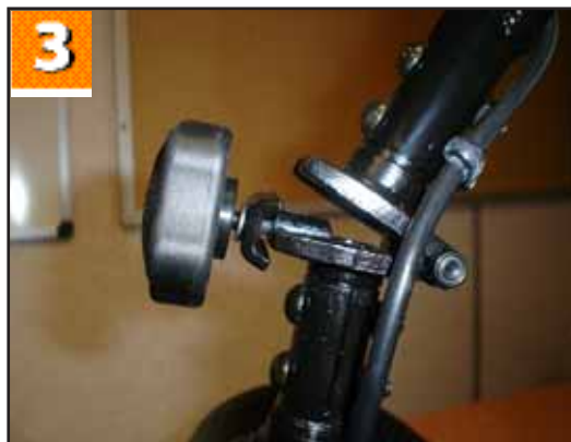
3. Lower the tiller by turning the black screw anti-clockwise.
