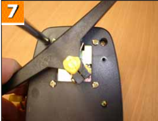
7. Using a small phillips screwdriver undo the 4 screws in the underside corners of the fascia control box.
