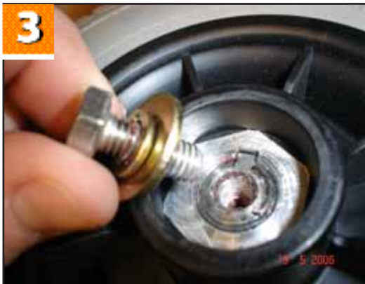
3. Remove the centre bolt, noting the positions of the spring washer and flat washer.
