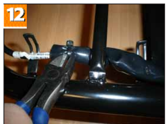
12. Cut the cable ties around the tiller connector protective sheathing and slide it away.
