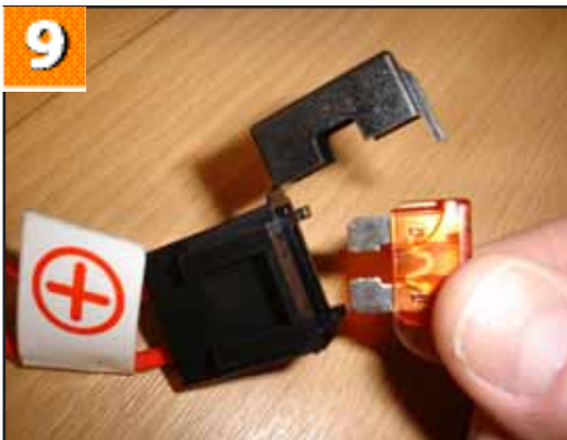
9. To access the 40A main blade fuses, flip up the lid on the fuse holder and pull the fuse out.
