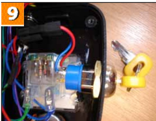
9. Shows the position of the key switch.
