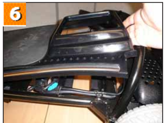
6. To release the tiller cable, remove the battery and lift the rear panel from the frame.
