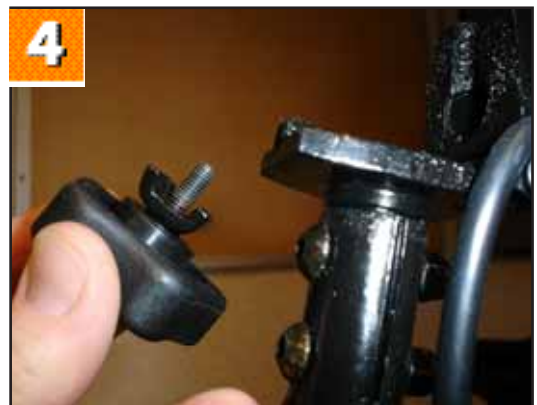
4. Shows the tiller locking screw and locking plate removed.
