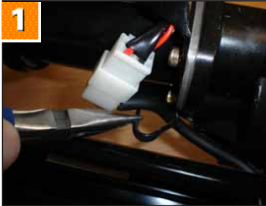
1. Using long-nosed pliers bend open the clip around the power terminal plug.
