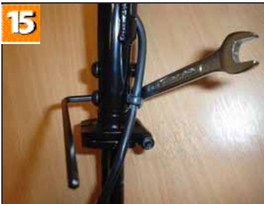
15. Undo the upper tiller mounting studs using a 4.00mm hex key and a 10.00mm spanner.
