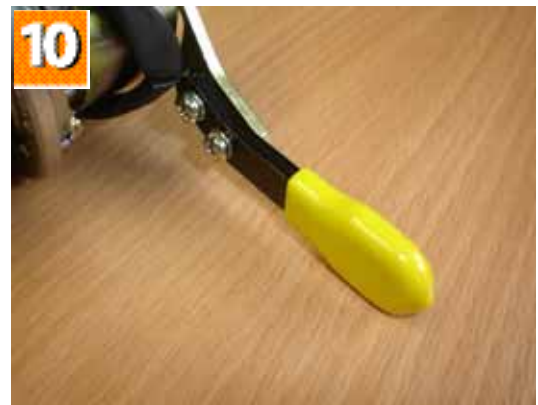
10. Shows the position of the freewheel extension lever held by 2 phillips screws.
