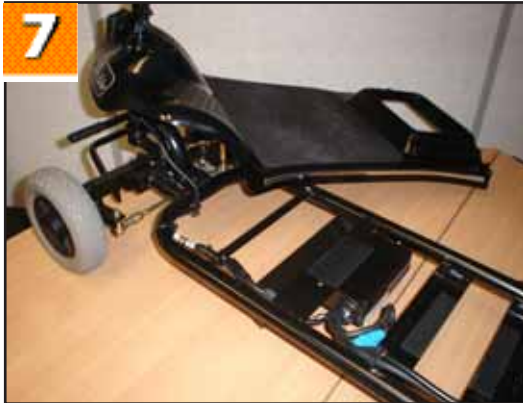
7. Move the panel over to expose the controller and main wiring looms.
