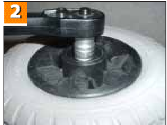
2. Undo the centre bolt using a 13.00mm socket.
