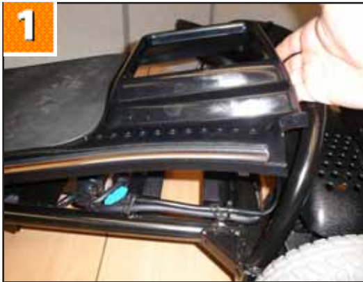
1. With the battery and tiller removed lift up the front panel from the rear pulling it off the frame clips and velcro.
