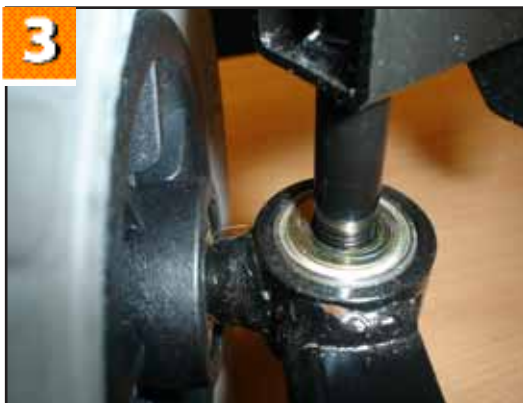
3. The stub axle may need to be carefully tapped with a nylon hammer and rotated to aid removal.
