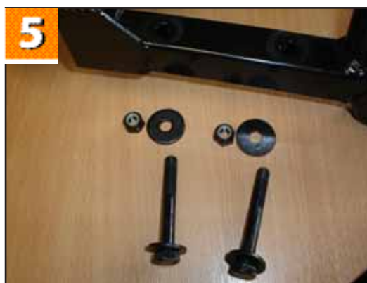
5. Remove the motor bolts carefully taking care not to damage the rubber mounts.
