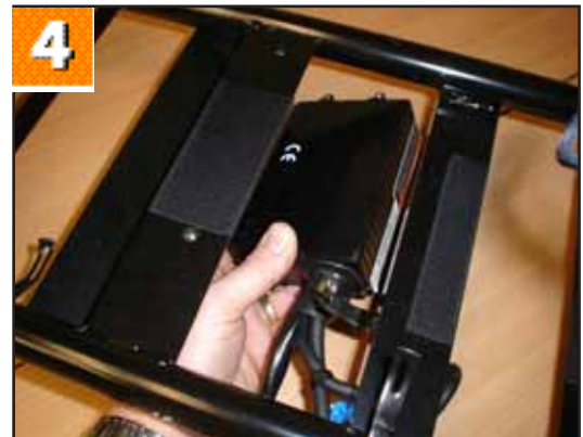
4. Lift out the main controller.
