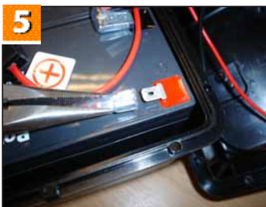
5. Use thin-nosed pliers to release the positive terminals....CAUTION! Take care not to short out the terminals.
