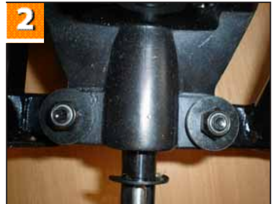
2. Location of 2 of the transaxle mounting bolts.
