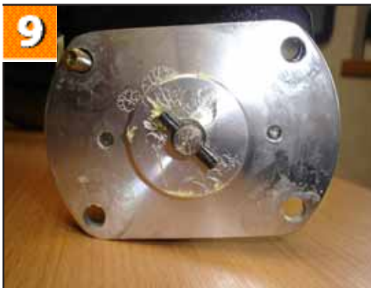
9. When refitting, the drive shaft coupling on the motor must line up with the drive shaft coupling inside the transaxle, (see over).
