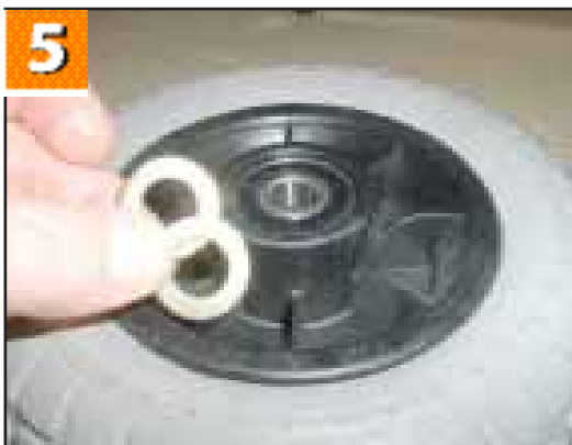
5. Note the number of shims behind the front wheels.
