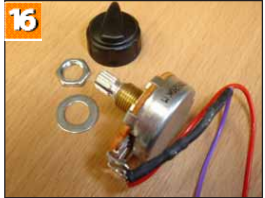
16. Shows the speed potentiometer.
