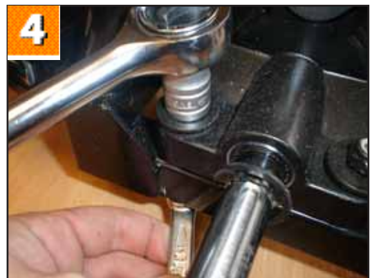
4. Use a 13.00mm socket/spanner to undo the four mounting bolts.
