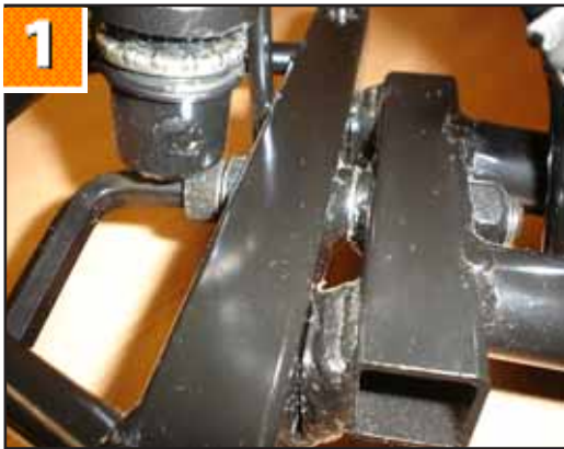
1. Using an allen key remove the bolt holding the front axle cross member.
