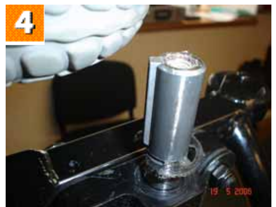
4. Carefully remove the wheel, taking care not to lose the Drive Key.
