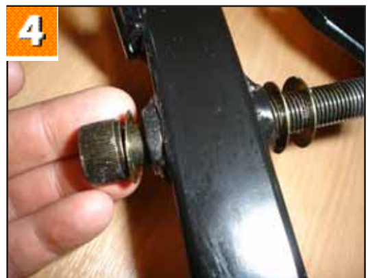
4. Pull cross member forwards remembering where the spacers are fitted.
