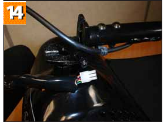
14. Carefully feed the tiller cable through the front panel and lift the tiller clear.
