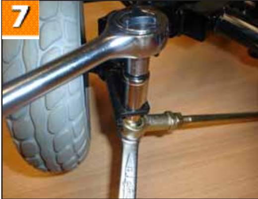
7. Use a 13.00mm socket & spanner to undo the other end of the steering link.
