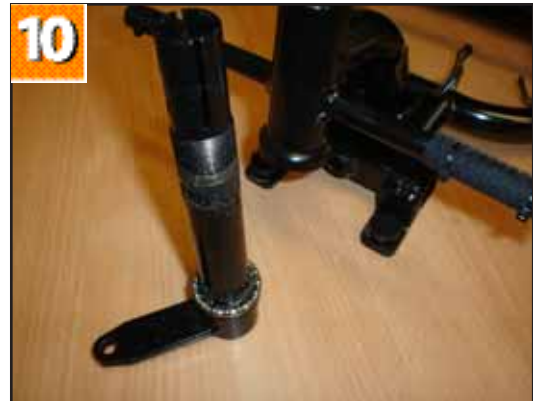
10. The steering head bracket showing the lower bearing in position.
