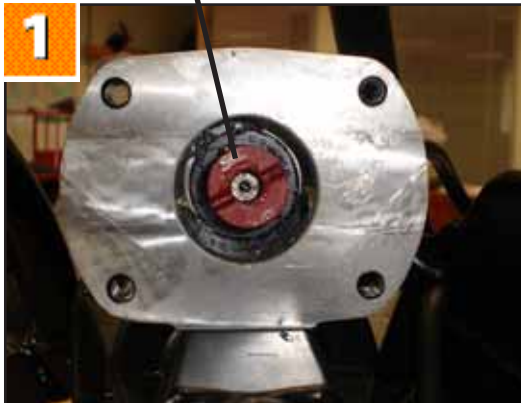
1. The drive coupling on the transaxle gearbox, must align with the motor drive coupling when reassembled.
