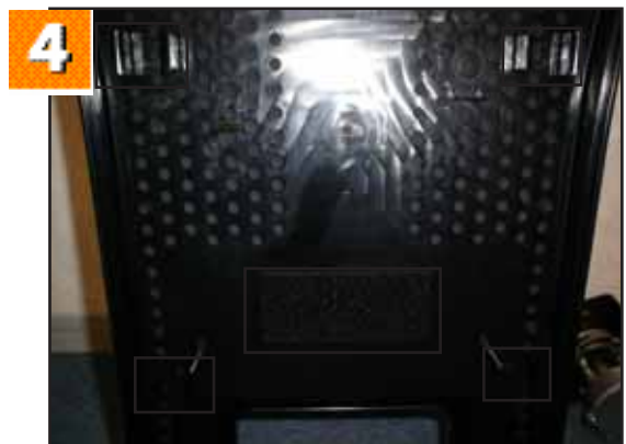
4. Shows the position of the front panel velcro (centre) and 4 frame clips (corners).
