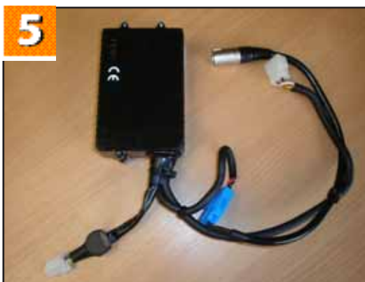
5. The main controller with tiller, motor and battery wiring shown.
