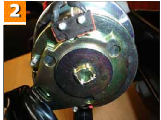
2. The micro-switch can then be accessed.
