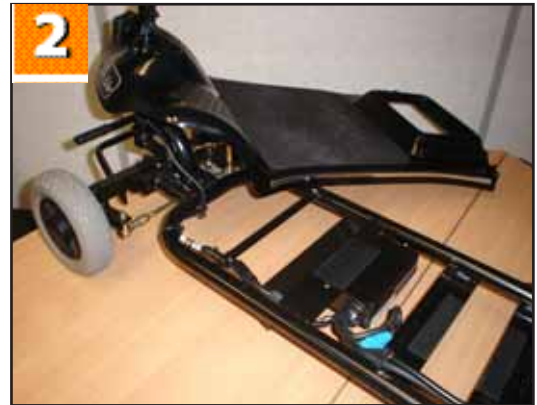
2. Move the panel away from the velcro and put in a position ready to lift clear.
