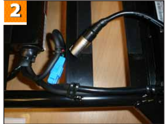
2. Using long-nosed pliers and wire cutters release the motor and power cable from their ties.
