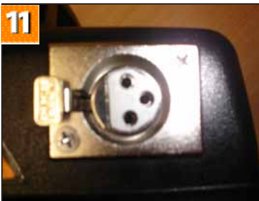
11. The battery connection / charging socket is secured by 2 small bolts.
