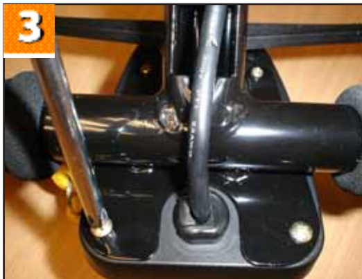
3. Undo the four screws in the bottom of the tiller fascia box.
