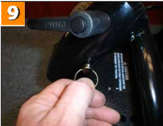
9. Hold the top of the Seat Stem & grab hold of the securing pin.
