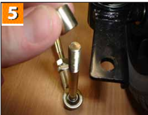
5. Lower the bolt out of the stub axle and remove the short spacer tube.
