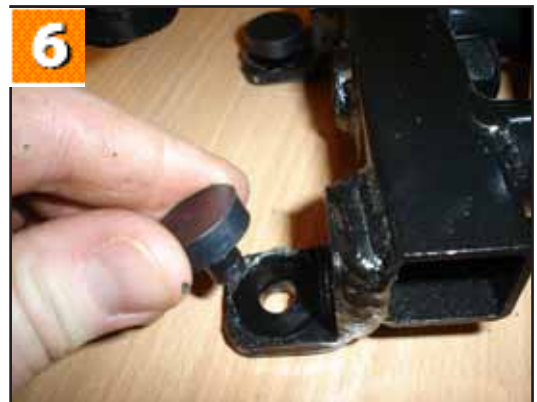
6. Inspect bump stop on frame for wear and damage, replace if necessary.
