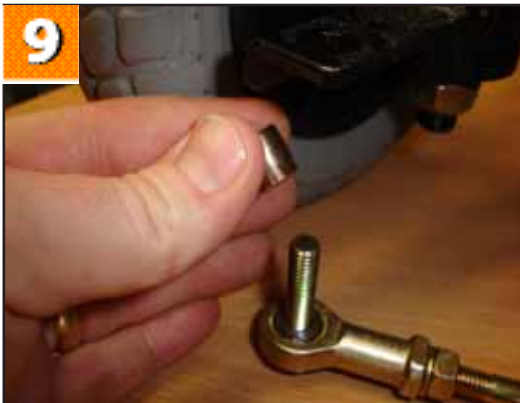
9. Lower the bolt out of the stub axle and remove the short spacer tube.
