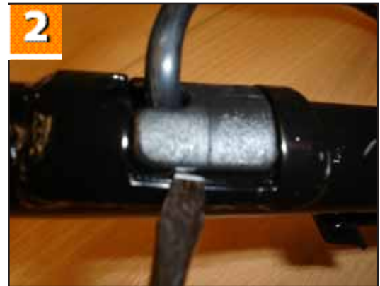
2. The Loom Clips can be removed with a flat screwdriver.
