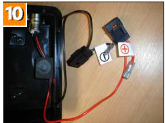
10. View of the battery main lead and socket.
