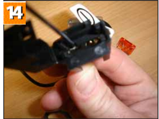
14. Using a small flat screwdriver remove the cable connecting the charge socket to the fuse holder.
