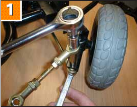
1. Use a 13mm socket and spanner to remove the other end of the steering link.
