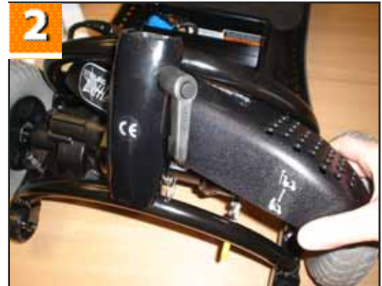
2. Slide out the rear panel by angling it slightly through the rear frame.
