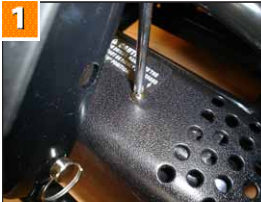
1. With the seat removed, use a phillips screwdriver to undo the rear panel retaining screw.
