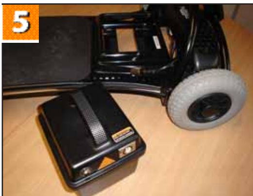
5. The battery box removed.
