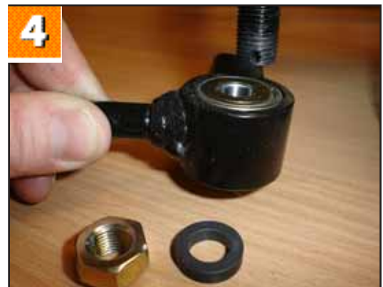
4. Remove the Stub Axle assembly Repeat the process for the other side.
