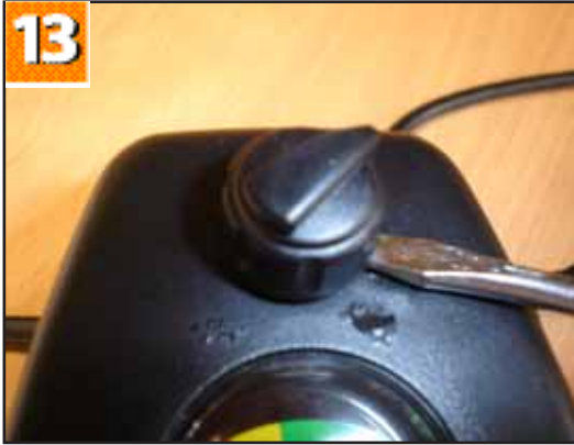
13. Using a flat bladed screwdriver carefully lift off the speed control knob.
