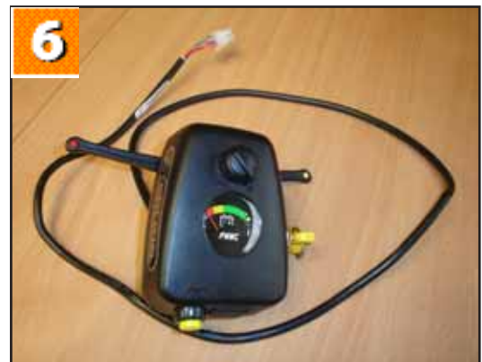
6. The tiller fascia control box.
