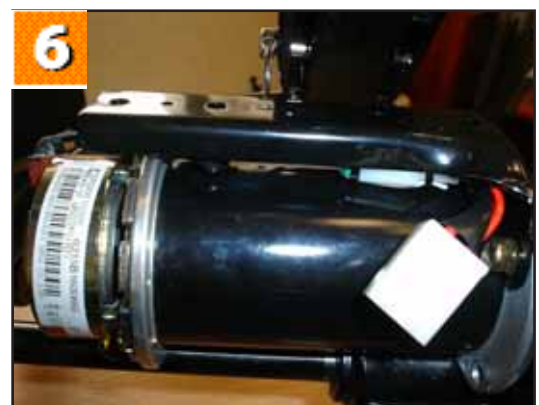
6. Shows the position of the rear panel bracket on the motor.
