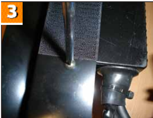
3. Unscrew the two screws visible from the top of the main controller. Note: Threadlock is used on these screws.
