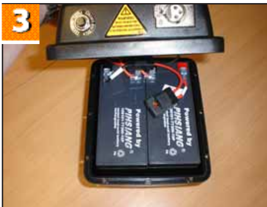
3. With the Battery Box on a flat surface, carefully lift the lid up.
