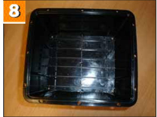
8. Shows the battery box base.
