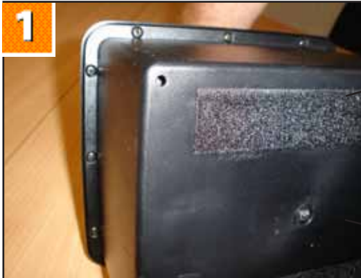
1. Shows the location of the 12 battery box screws beneath the lip of the battery box.
