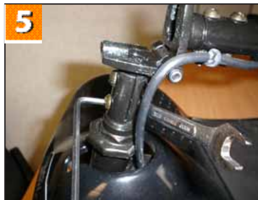
5. Undo the lower tiller mounting studs using a 4.00mm hex key and a 10.00mm spanner.
