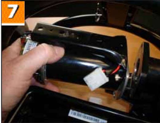
7. Gently ease the motor away from the transaxle.
