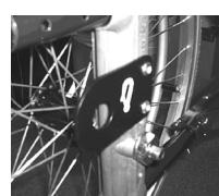
Position of the rear wheelchair tie down restraint and the tie down label on the wheelchair.
