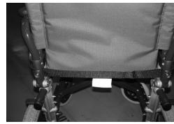
**⚠** It is important that the belt is routed around the back of the wheelchair. The buckle end can be fed between the armrest and backrest.
