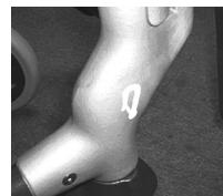
Position of the front wheelchair tie down restraint and the tie down label.
