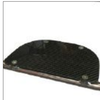
Tubular footrest welded into frame with Carbon plate
