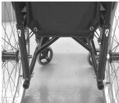
Position of the rear wheelchair tie down restraint and the tie down label on the wheelchair.
