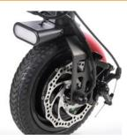
LED-light, Fender (accent colour red) and disc-brake (pictured on EMF070085 Drive wheel 8,5", solid tyre)
