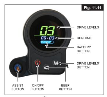
On/off method: press **(b)** short, beep once, to turn the R10 on successfully; press **(b)** long, beep once, to shut down the R10 completely.
