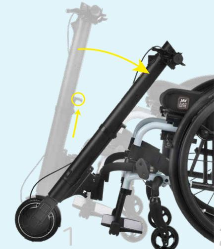
Pull and hold the docking release lever on the main tube. Now pull the handlebar gently backwards/downwards.
