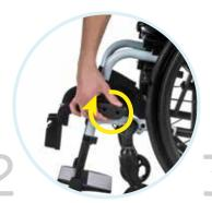
Now rotate the tommy screws of the clamps in a clockwise direction until they are hand tight and the intermediate sub-frame is securely held in the clamps. Take the pull device and insert the docking pin ends into the central bracket of the subframe.
