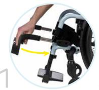
Insert the subframe into the docking clamps.
