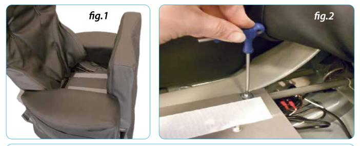
To set the seat depth, first pull the seat cushion forward as shown in **fig.1** to locate the two locking screws at the back of the seat plate **fig.2**.
