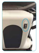
On single function power chairs simply activate the tilt in space by pressing the rear rocker switch on the back moulding, until the desired angle is reached.
