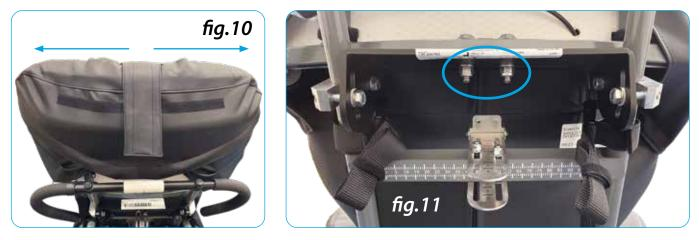
The headrest can be offset to the left or the right if required **fig.10**. Remove the back shell as previously described on page 8 and loosen the two nuts underneath the black bracket as shown in **fig.11**. Reposition the headrest as required and tighten the nuts to lock in place.
