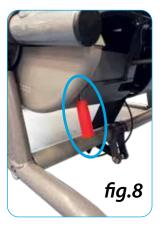
To raise the manual leg rest simply lift to the required angle. To lower it locate the red handle **fig.8** behind the cushion on the left side of the chair. Lift the leg rest slightly whilst pulling the lever and then lower to the required angle. It will lock in to place when the lever is released.
