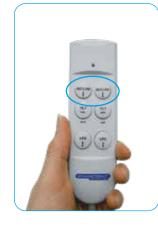
The angle of back elevation can easily be altered on the powered chair simply by pushing the buttons on the handset as shown above to alter the User's recline angle. The green light on the handset will illuminate during operation.
