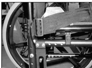
**⚠ It is important that the belt is routed around the back of the wheelchair. The buckle end can be fed between the armrest and backrest.**
