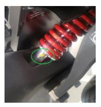
**Firm Suspension setting**: The Firm Suspension setting is what we have historically manufactured to date on Q400 M and Q500 M. The former ride setting is recommended for clients with Lift and Tilt and with a MUW of over 100KG on Q400 M and 75Kg on Q500 M. The stiffer setting in addition to higher client and chair configuration rate provides excellent performance, stability and traction.
