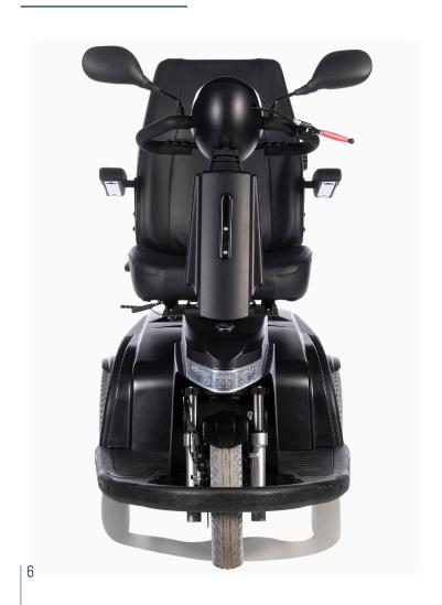
Brake lever in red for better and faster recognition (for Elite<sup>2</sup> Plus & Elite<sup>2</sup> XS)
