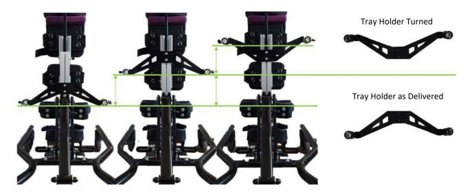
Changing of the tray bracket is simple and easy to do; just loosen the bolts fixing the metalwork to the central extrusion, slide off the extrusion, flip the bracket over, slide back into the desired position and then tighten the bolts. Spare part numbers will remain the same and can be retro fitted onto older models.
