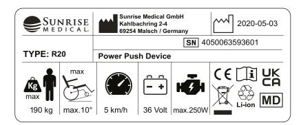
As we are committed to continually improving the construction of our wheelchairs and pushing devices, product specifications may vary slightly from the examples illustrated. All weight/dimensions and performance data is approximate and is provided solely for guidance.
