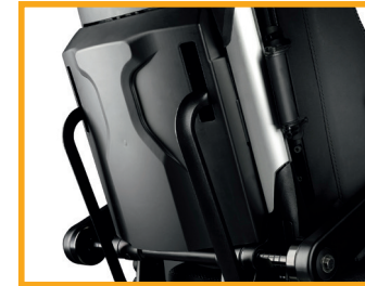
Powered Recline with 100 mm Anti-Shear, 90°-150° Its patented unique mechanism enhances ski protection and allows the positioning element and even chin control to stay in place during full recline operation.
