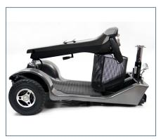
The tiller can be safely secured in position for transporting.
