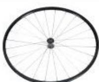
Rear wheel, Lightweight, 24 spokes, straight spokes
