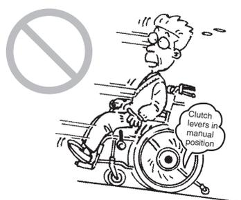
**If you switch the clutch levers to the power drive position while traveling in the manual drive, brakes are applied to the rear tires. This abrupt braking can cause your body to plunge forward or damage the wheelchair.**
