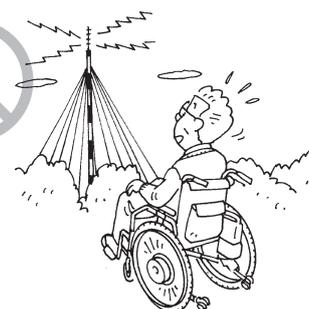
The weak electromagnetic waves emitted by the iXpress may affect other electronic devices, such as automatic doors and the anti-theft systems of stores. In this case, turn off the power and operate the wheelchair using the assistant operations or manual operation.
