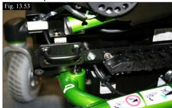
4. INSTALLEZ LA FIXATION D'ARRIMAGE ARRIERE, (Fig. 13.53).
