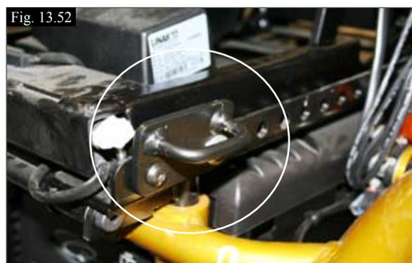
3. INSTALLEZ LA FIXATION D'ARRIMAGE ARRIERE, (Fig. 13.52).
