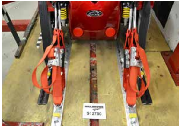
Rear tie-down point on the wheelchair Caution: two straps on each side!
