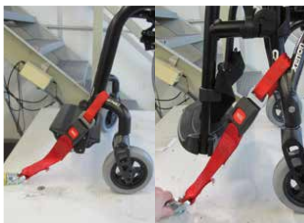
Front tie-down point on the wheelchair Left: Xenon 2 ; Right: Xenon 2 SA
