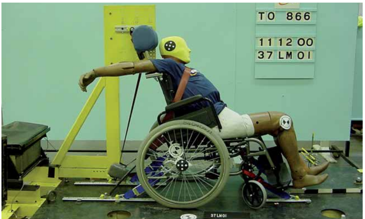
Wheelchair secured on the rails, after impact
