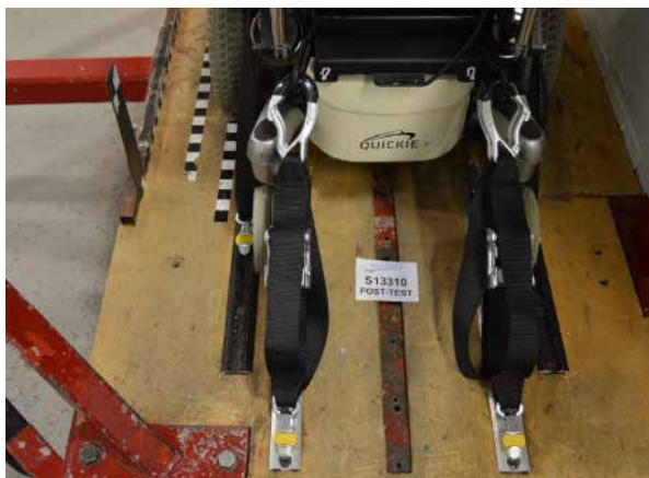
Rear tie-down point on the wheelchair Caution: two straps on each side!
