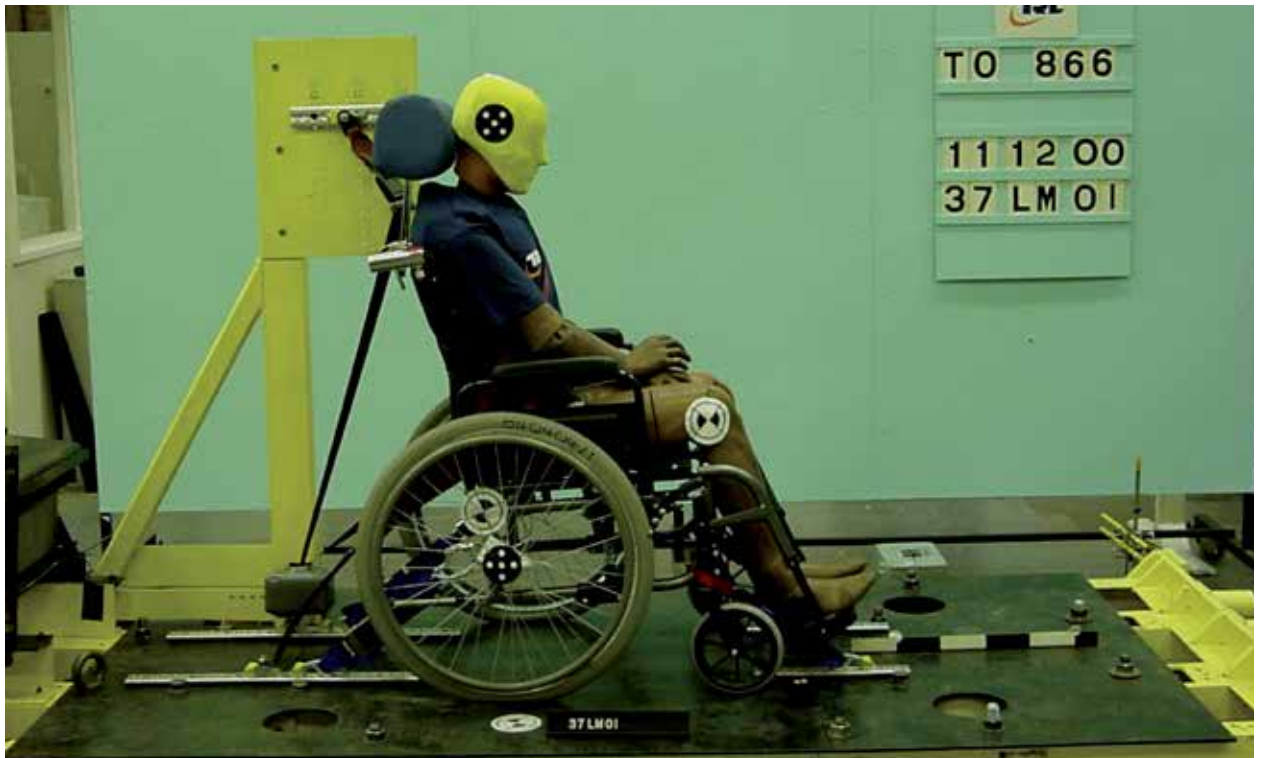
Wheelchair secured on the rails, before impact
