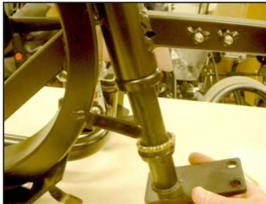
10. With the top bearings removed, lower the steering head to expose the bottom bearing race.
