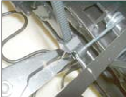
18. With the fulcrum bolt removed, cut the first tie wrap.
