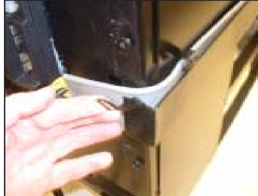
14. Start by undoing the wire clip at the rear end of the loom.
