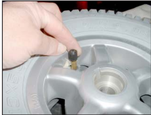
2. Remove the valve dust cap and deflate the tyre as previously described.
