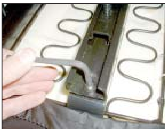
9. Slide the seat rails forward to expose the bottom bolts and use a 5.00 mm hex key to undo them.
