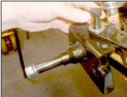
9. Use care when lifting the pivot bolt out, as there are bushes and spacers which can fall out of the assembly.
