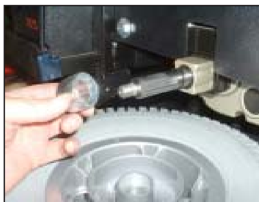
11. Remove the spacer. Note that there is a rebate cut into the end of the inside face of the spacer.
