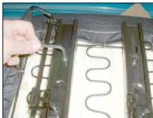
11. Undo the top two bolts.
