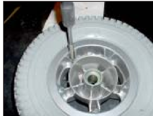
4. Remove the five recessed rim studs using a 4.00 mm hex key/driver.
