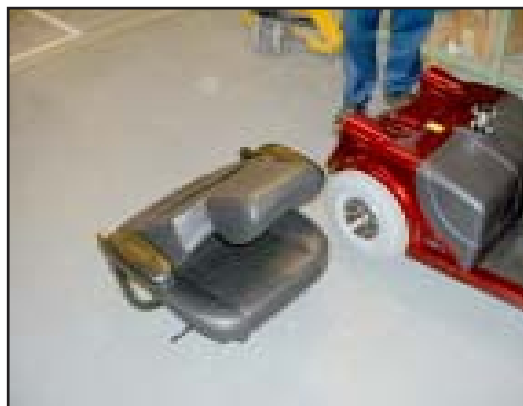
5. The complete seat assembly removed.
