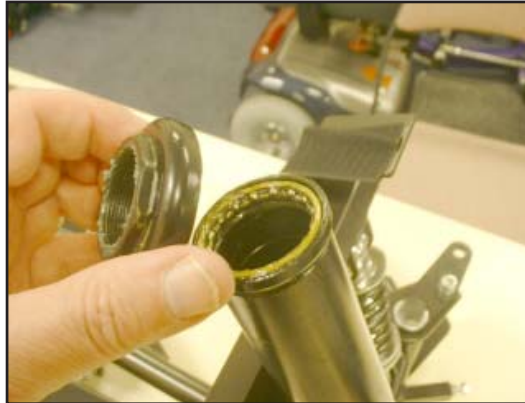
8. Removing the nut, exposes the top steering bearing race.
