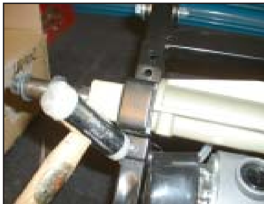
12. Some studs may require tapping out with a soft face hammer.
