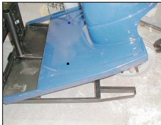
4. Lift the Footboard clear of the frame.
