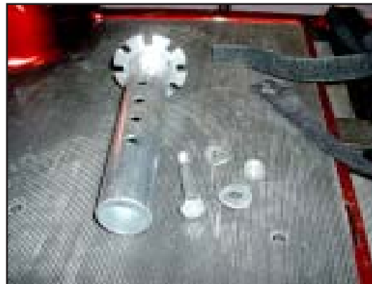
6. Lift the seat stem out. Note the height positioning holes in the seat stem.
