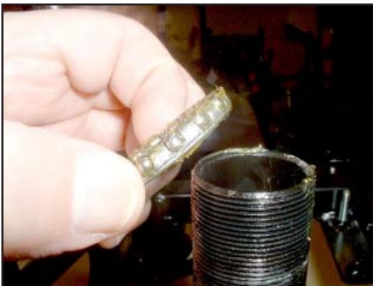
11. Feed the lower bearing race, up and over the top of the steering head.
