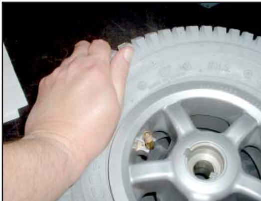
3. Squeeze as much of the air out of the tyre as is possible. At this stage, use a non-corrosive releasing agent between the tyre & rim.
