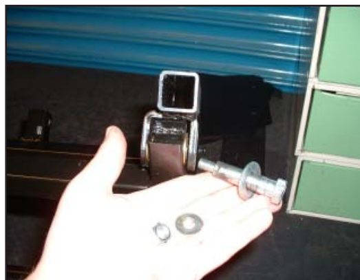
22. Take extra care when loosening/removing the pivot bolts as the frame can drop down suddenly.
