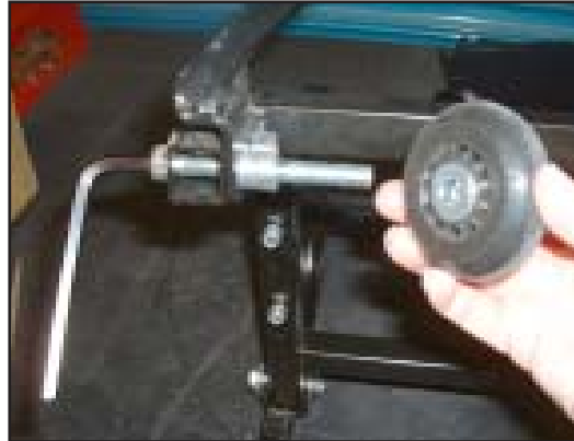
14. Slide the stabiliser wheel off the axle stud.
