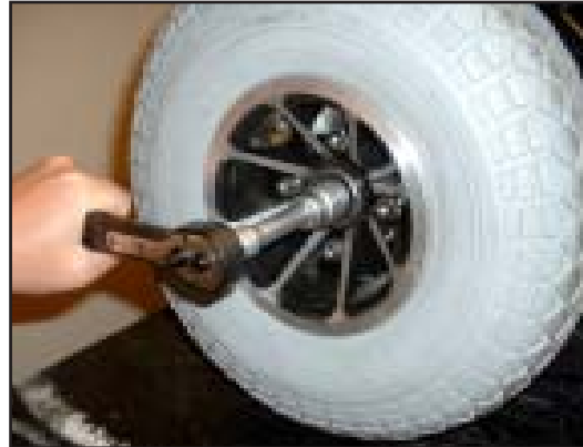
2. With the wheel on the ground, use a 19.00mm socket to loosen the centre self-locking nut
