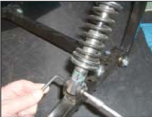
3. The struts are secured by two concentric studs. Use two 5.00mm hex keys/drivers, to undo them.
