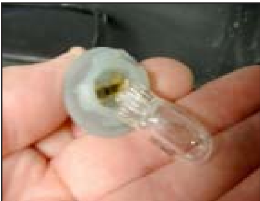
9. Carefully pull the bulb out of the holder. All rear bulbs are 24V - 5W Capless type.
