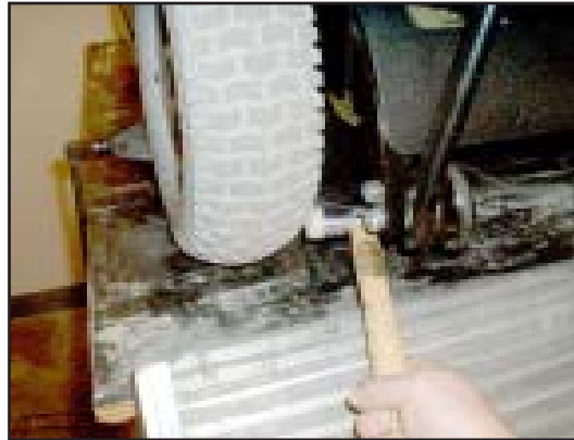
8. Because the rear wheel is keyed to the drive shaft, a small amount of force may be carefully applied to loosen the wheel.
