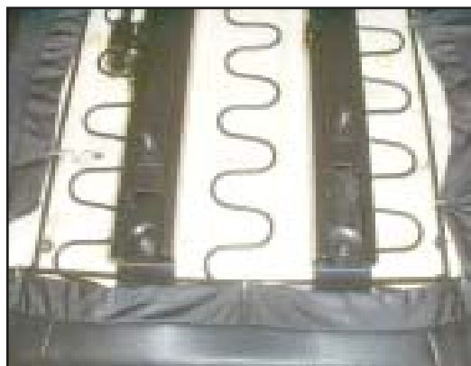
8. There are four hex bolts securing the two seat rails top and bottom.
