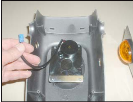
1. The Horn or Audible Warning Device, (AWD), is located on the Tiller Front Panel.
