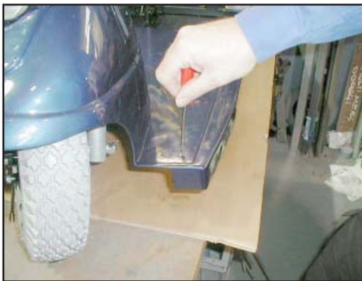
1. Unscrew the left-hand front self tapping screw
