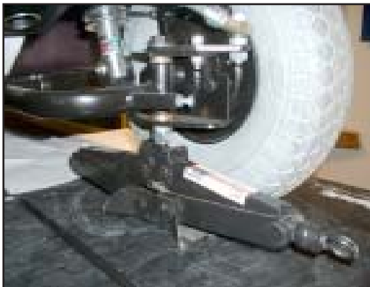
3. Once the centre nut is loosened, raise the wheel using a jack or axle stands/blocks.
