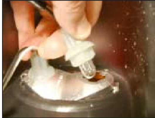
8. Twist and turn the holder to remove it from the back of the light cluster.
