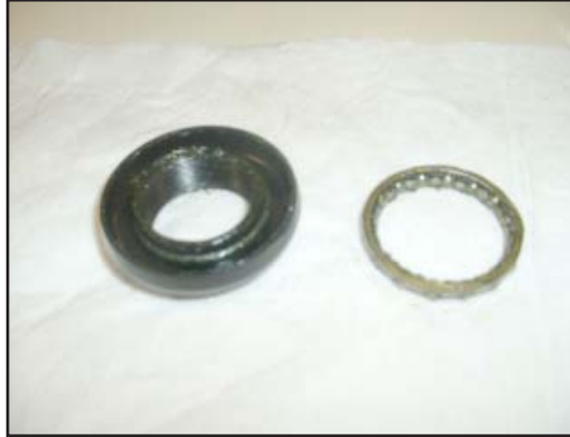
8. Steering top bearing and retaining nut.
