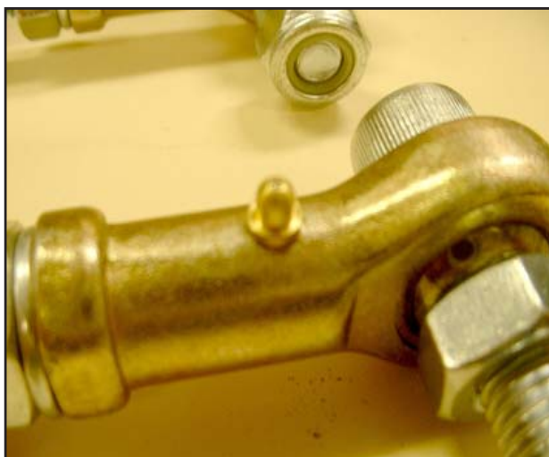
11. Each end of the steering rods have grease nipples to aid the application of lubricant.
