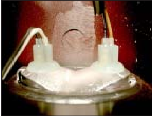
7. The two rubber bulb holders at the back of the light cluster.
