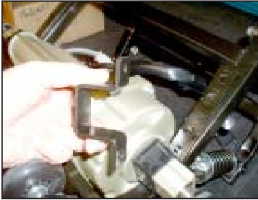
13. Lift the “U” brackets off the transaxle.
