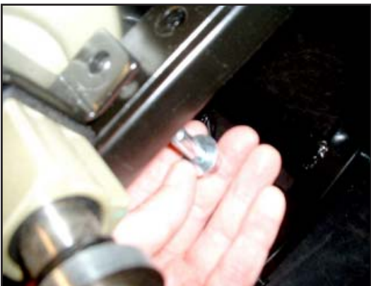
11. Some studs may drop out of the frame quite easily.
