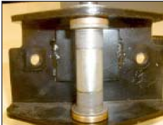
16. View of the bushing order; Brass Bush, Sleeved Bush, Spacer, Sleeved Bush and Brass Bush.
