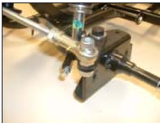
18. The remaining stub axle is a "mirror image" of the previous one and is removed using the same process.
