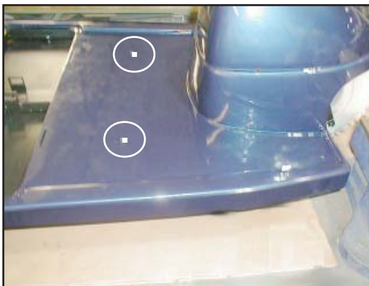
3. Undo the two self tapping screws at the rear of the foot board.
