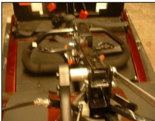
10. Use a 12.0mm socket & 10.0mm spanner to undo the Tiller Bracket bolts.
