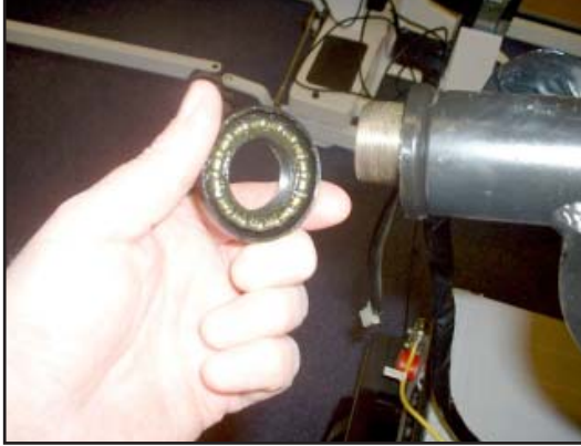
7. The top steering bearings usually come away with the nut.
