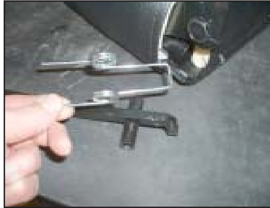
20. Remove the spring by pulling the two coiled sections off the lever fulcrum.
