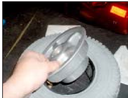
6. Lift the outer rim from the tyre & proceed as before to remove the tube. Note that the outer rim has an integrated hub.
