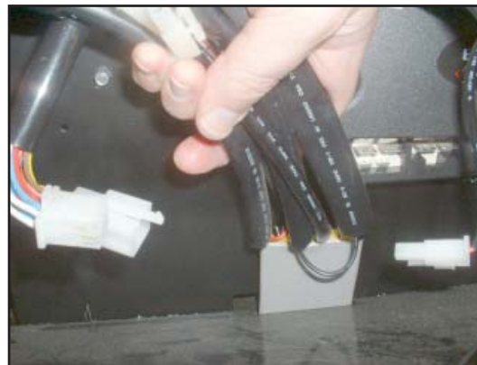
6. Make sure the loom is free of cable ties and connections.
