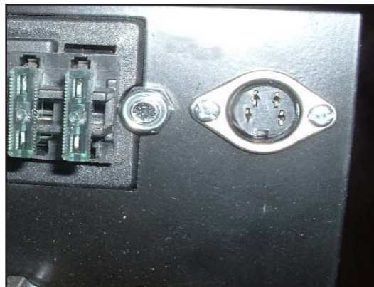
12. The programming socket is located next to the fuse panel on the Elite only. The Onyx is programmed directly into the Egis main control box.
