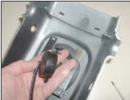
3. Undo the screw to remove the Horn, (AWD).
