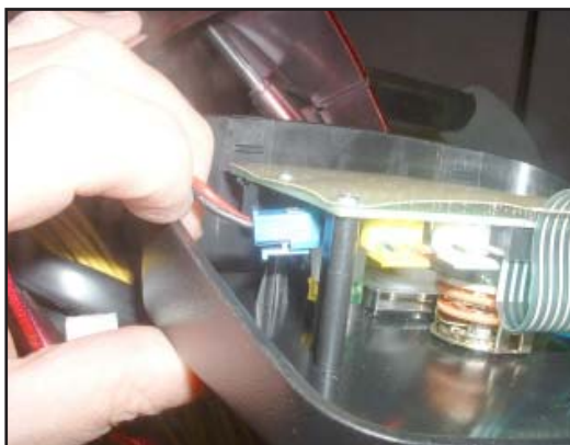
8. Use the same procedure to remove the blue plug.
