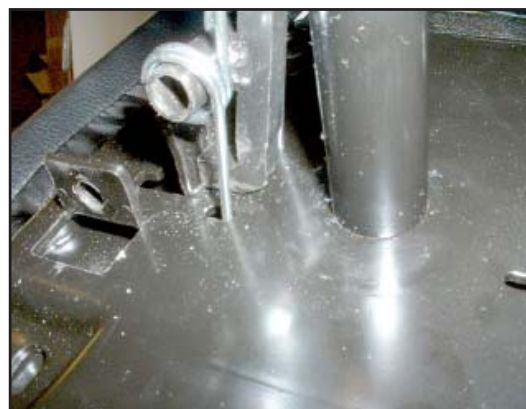
24. Squeeze the two ends of the spring into the two holes whilst holding the lever vertically. The angled end of the lever should face away from the seat post.
