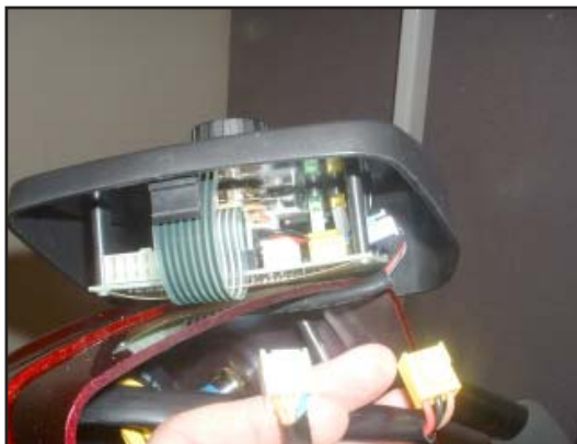
7. Remove the two plugs.
