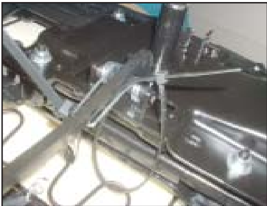
15. Use a second tie wrap, adjusted slightly looser to catch the spring if it flies up.
