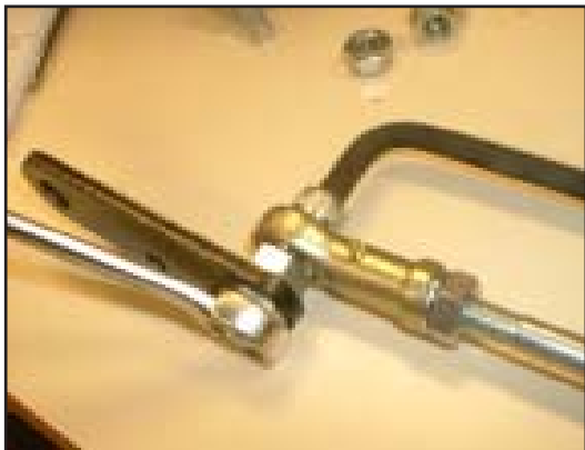
9. If the stub axle has been removed before the steering rod, the stub axle pivot bracket will have to be removed from the steering rod.
