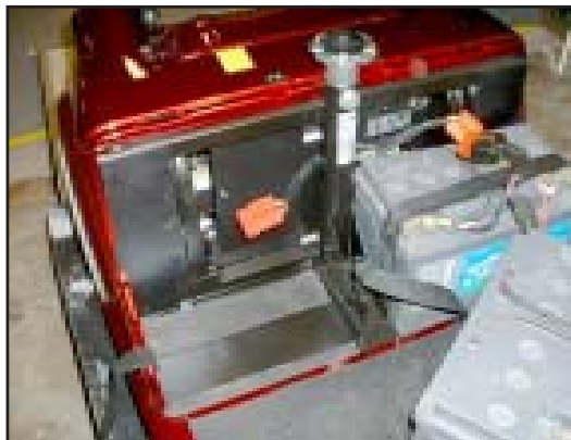
11. Remove the batteries one at a time.
