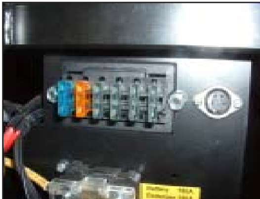
10. There are six blade fuses in total, each have the rating in amps marked on the body.
