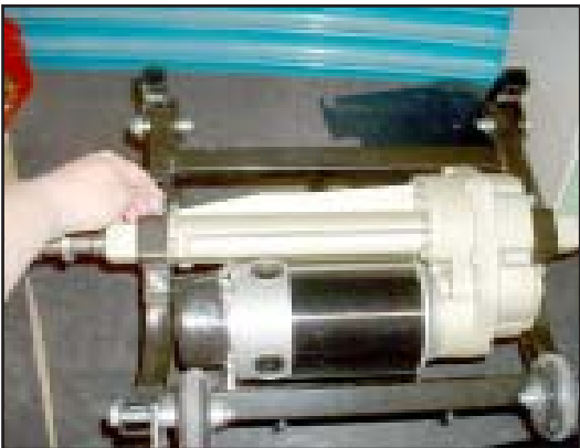
9. Remove the nuts using finger pressure.
