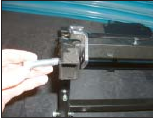
19. Remove the studs on both sides.
