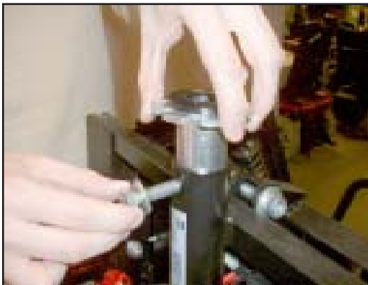
5. Hold the top of the seat stem to prevent it from falling when the bolt is withdrawn.
