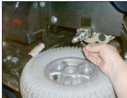
10. Remove the drive key.
