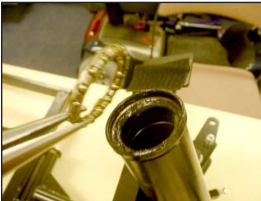
9. Use thin nose pliers to lift the top bearings out.
