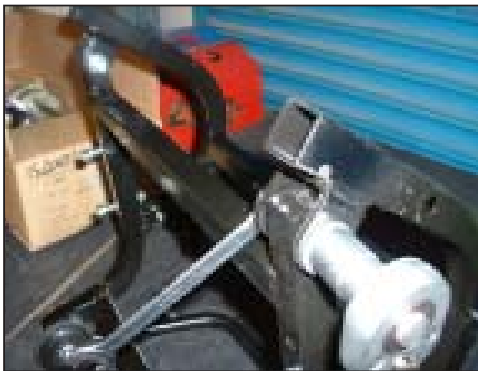
21. Use a 17.00mm socket and a 13.00mm spanner, to undo the rear frame pivot bolts.
