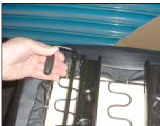
10. Depress the seat slide and slide the rail back to expose the top two bolts. Note that the other rail slides freely.
