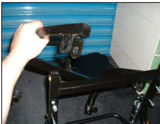
23. Lift the two halves of the frame apart.
