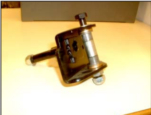
15. The Stub Axle assembly.
