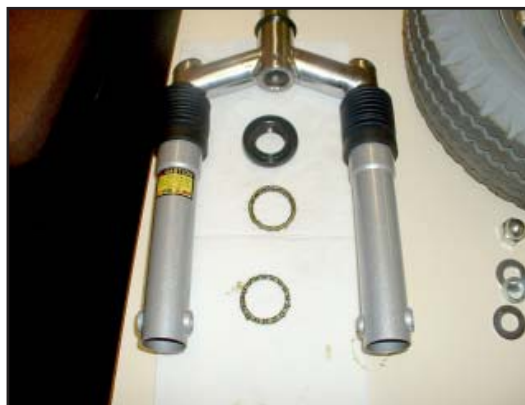
11. View of the Steering bearings, retaining nut and Front Fork assembly.
