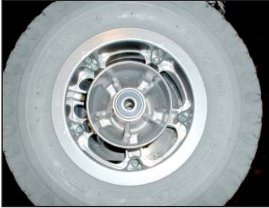
1. The five rim studs are accessed from the back of the wheel.
