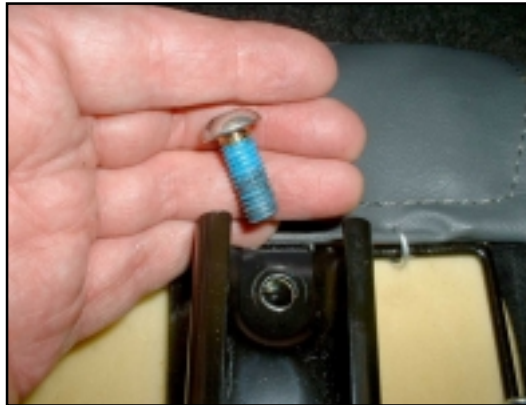
16. The blue thread-lock is the reason the studs are so tight.
