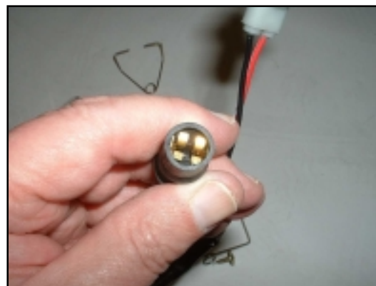
12. Make sure that the copper terminals do not touch as this will cause a short circuit. After changing bulbs, always try the lights prior to returning to the customer.
