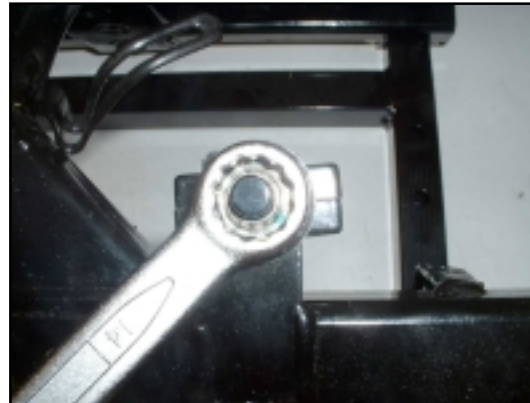
2. and use a 14.00mm spanner to undo it.
