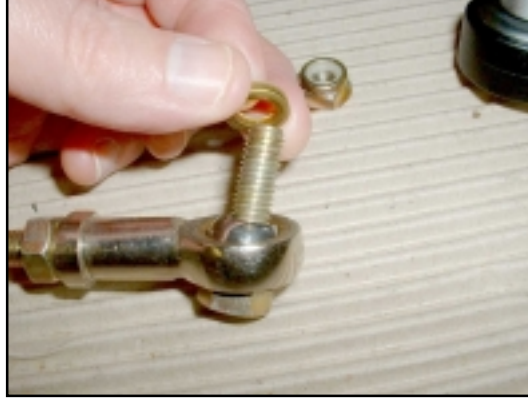
8. Lift the small spacer off.
