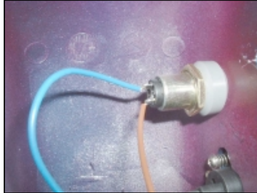
20. The two wires on the back of the Key Switch, have to be de-soldered for removal and soldered back on.
