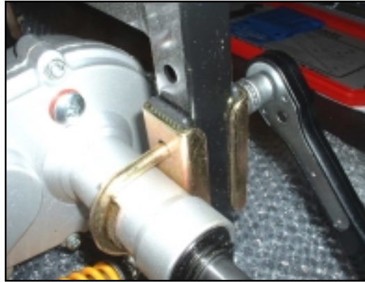
8. Use a 13.00mm socket to undo the nuts on the "U" bolt side of the drive train.
