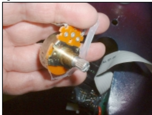
18. Withdraw the Pot. Note that there is a low tack glue used on the Pot face. It is advisable to use a low tack compound or a star washer when refitting. This prevents the Pot body turning against the securing nut.
