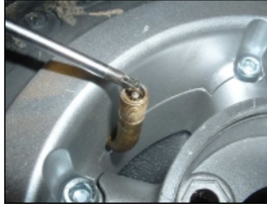
2. Use a small screwdriver or similar, to depress the valve pin and let out as much air as possible.
