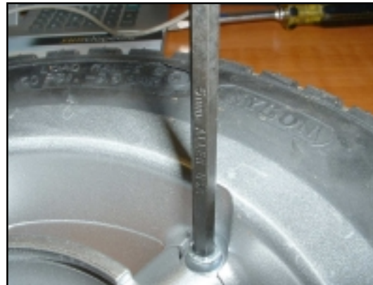
18. Use a 5.00mm hexagon wrench to undo each of the studs. When re-tightening, use the sequence shown above.
