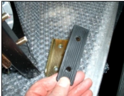
10. Remove the rubber gaiter.
