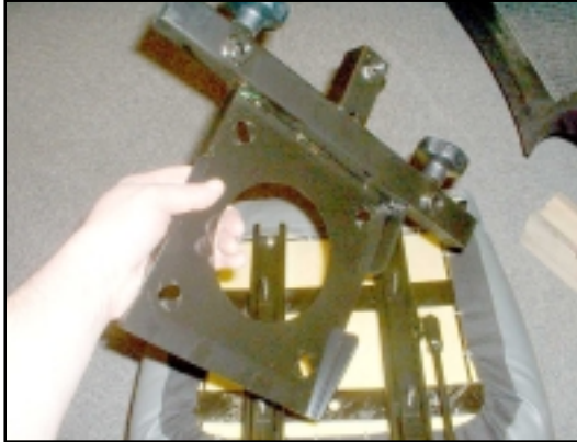
13. Lift off the armrest adjuster bracket.
