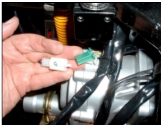
3. There are two White plugs mating to one Green socket and one White socket. On the other side there is the same, but it is a Yellow socket.
