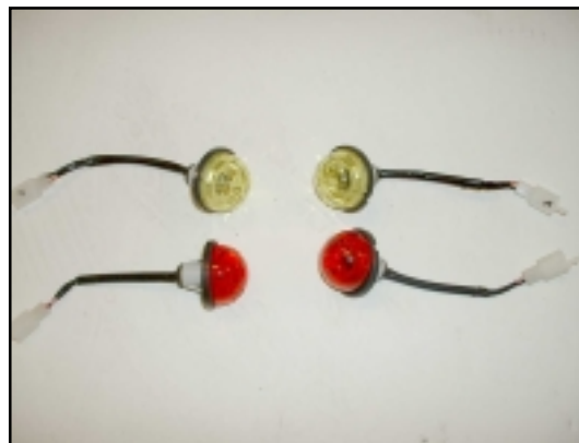
10. Note that the rear tail & indicator lights are sealed. If a bulb blows, the complete assembly has to be changed.
