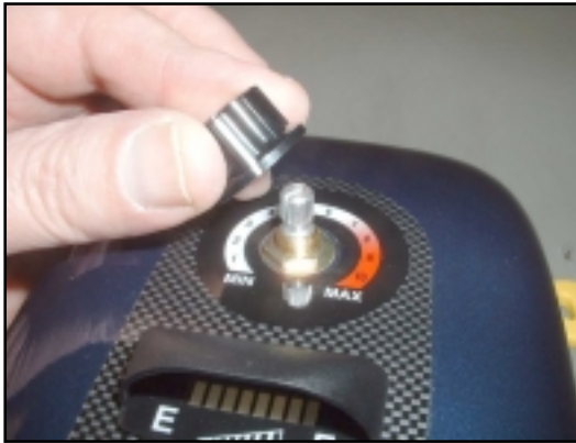
15. Turn the Preset Speed pot to either min. or max, then remove the pointer knob by pulling it upwards. When refitting, align the pointer to the chosen min. or max position.
