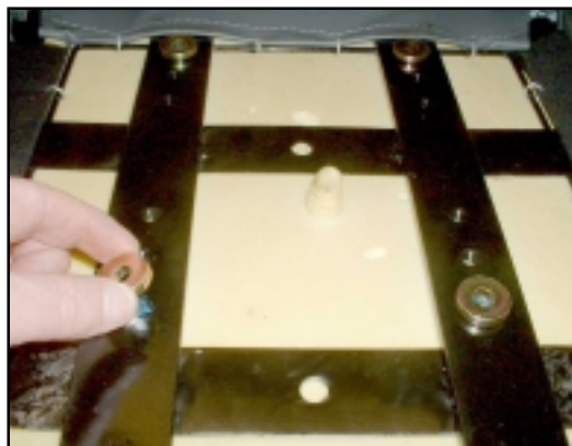
23. Finally remove the four spacer washers.
