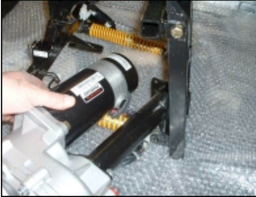
13. Retract the Drive Train Assy. Use caution as this part is heavy
