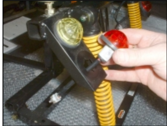
8. Withdraw the light assembly.
