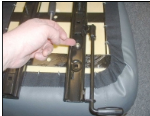
18. Once the slides are pushed back, the other two studs are exposed.
