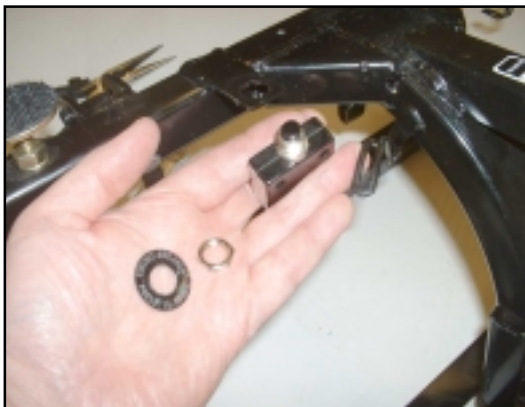
3. Check that there are no broken terminals or cracks in the Power-breaker body
