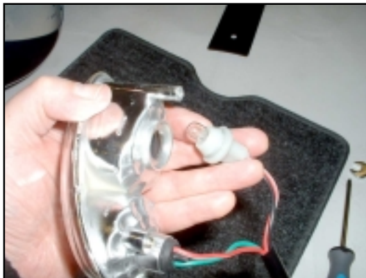
10. Pull the plastic bulb mounts out of the cluster body, to access the bulbs.
