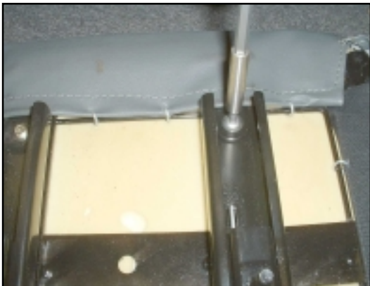
15. Use a sturdy 5.00mm hex wrench to undo all four studs. Note that these are firmly held & some force is required.
