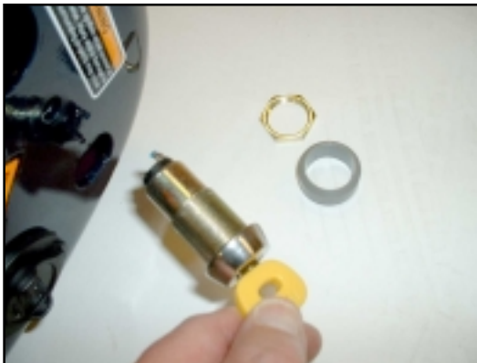
23. Withdraw the Key Switch.
