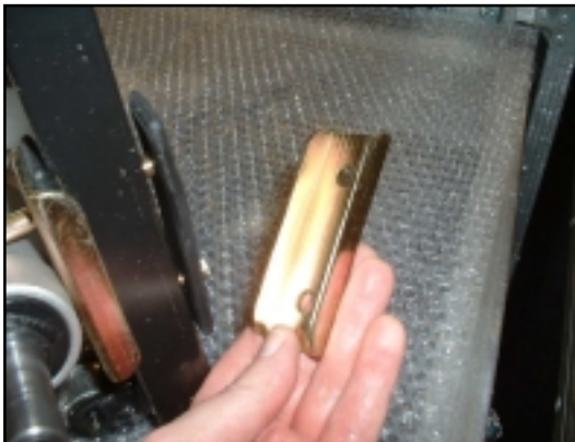
9. Remove the brass bracket.
