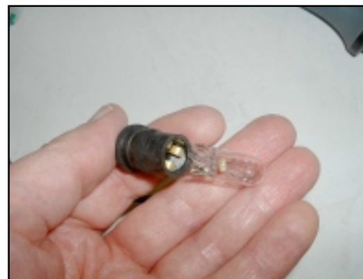
11. To release the bulb, gently pull on the glass envelope. Take care as the bulb is cap-less and the glass can break.
