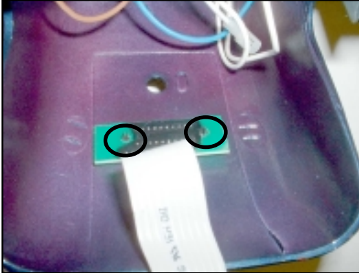
19. Press out the two plastic pop rivets to remove the Bar Graph PCB.
