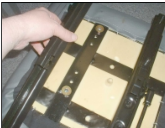
21. Once the studs have been removed lift off the seat slide.
