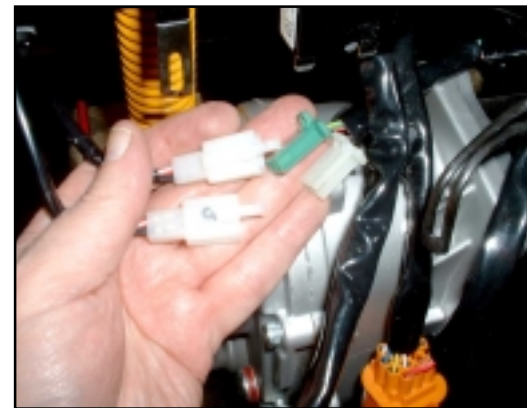
4. Mark the White plug which goes to the Green socket, (Yellow on the other side), to aid reassembling. Do this before disconnecting them.
