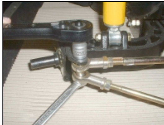
10. Use a 13.00mm spanner/socket to undo the bolt and self-locking nut on the other Stub Axle.
