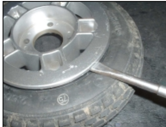
4. Press down on the tyre with the ball of the hands and use a tyre lever to gently lift the rim away from the tyre.
