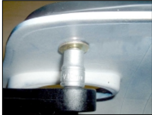
2. Use a 10.00mm socket to undo the nut. When refitting, do not over-tighten.
