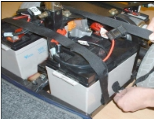
3. Undo the two velcro straps that secure the batteries.
