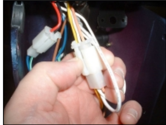
8. Unclip the 3-way molex plug located behind the Tiller Panel.
