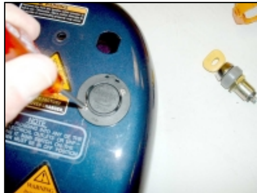
24. Use a small X-head screwdriver for the outer screws on the Charger Socket.
