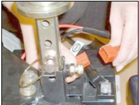
4. Disconnect the Red & the Black battery plugs.
