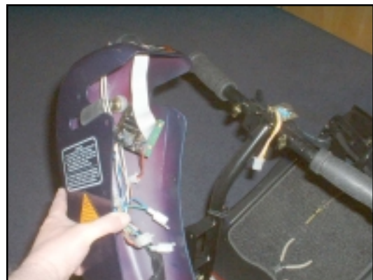
12. Lift the Tiller Panel away from the handle bar assy.
