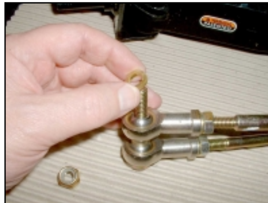
12. Lift the small spacer off the bolt.
