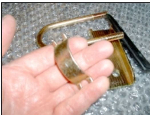
12. Be careful not to lose the arched sleeve that is positioned at the inside top of the "U" bolt.
