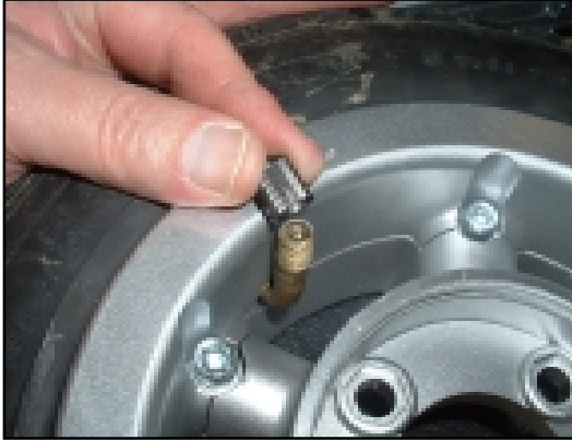
1. Remove the valve dust cap.
