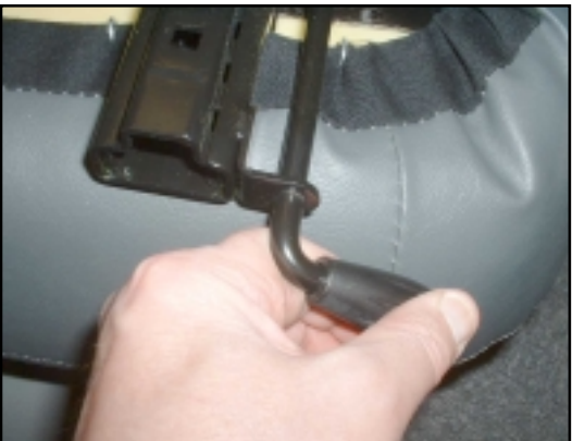
17. Press the seat slide lever down to move the slide to the rear. The other slide can be pushed back freely.
