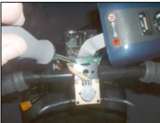
11. Undo the small brass screws that secure the Throttle PCB to the handle bar assy.
