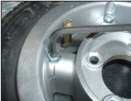
3. Use a 5.0mm Hex Key, to undo the five rim studs.
