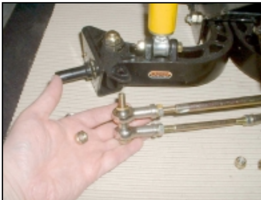
11. Drop the rods away from the Stub Axle.
