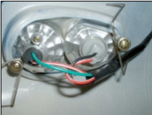
3. The Front Light Cluster is held in place by mounting springs and screws.
