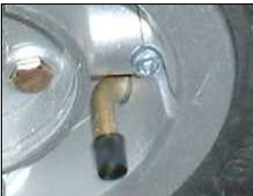
17. Before undoing the five wheel rim studs, be sure to deflate the tyre through the air valve.
