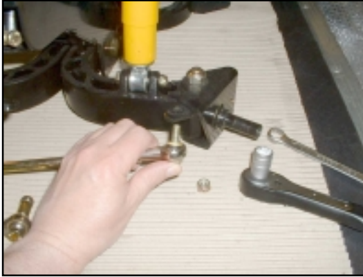
7. Drop the rod out of the Stub Axle.
