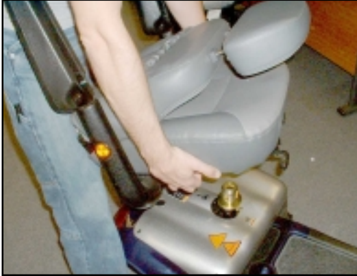
1. To remove the batteries, lift the seat off.
