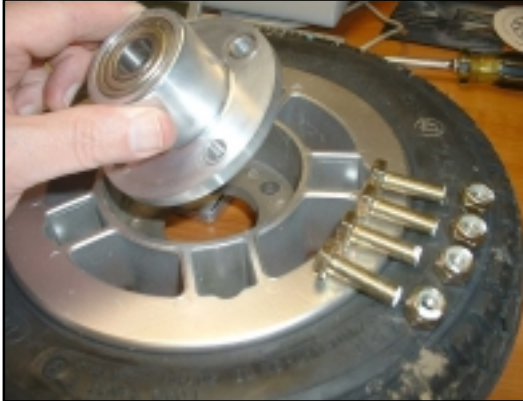
13. Remove the bolts & carefully lift out the wheel hub.
