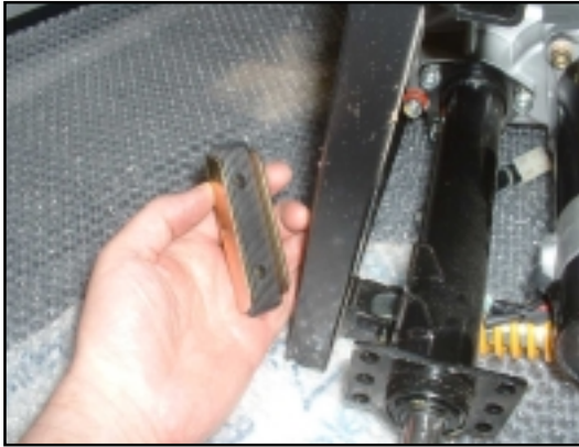
7. Remove the brass bracket complete with the rubber gaiter.
