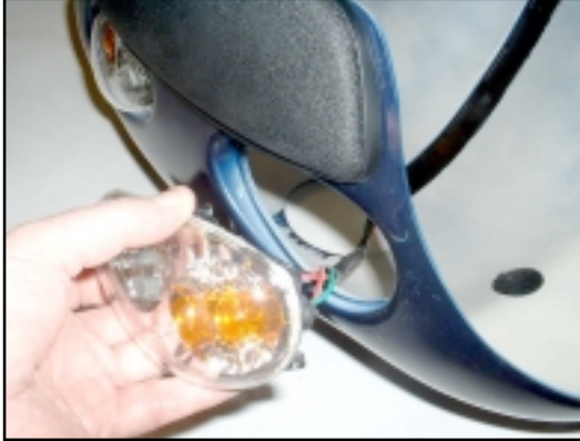
7. Withdraw the Front Light Cluster from the front of the panel.
