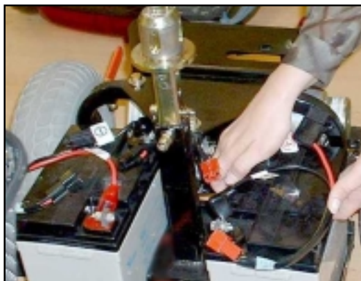
5. Carefully lift the batteries out.
