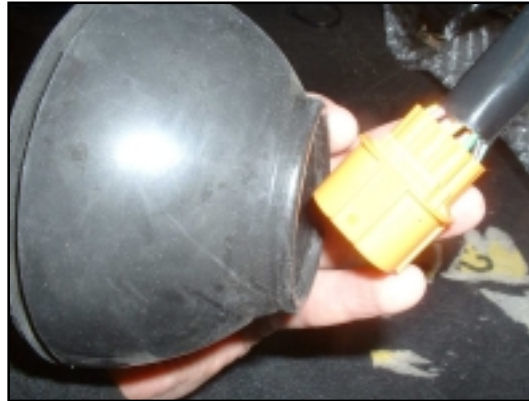
2. Pull the Rubber Gaiter off the Main Loom.
