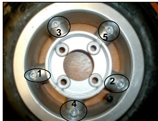
16. Location of the five wheel rim studs. The numbers indicate the re-tightening sequence
