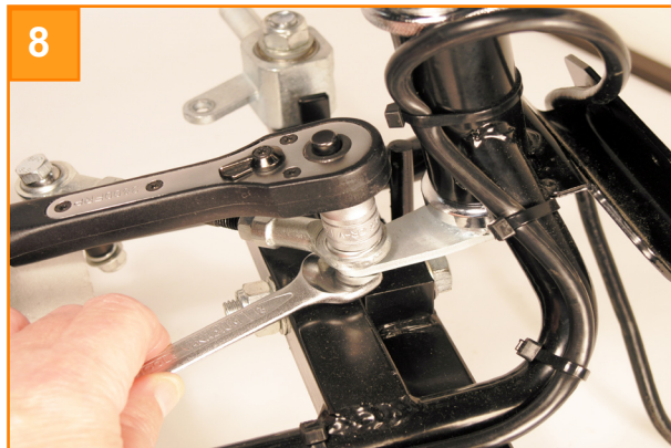
Use a 13.0 mm spanner/socket to undo the bolt.
