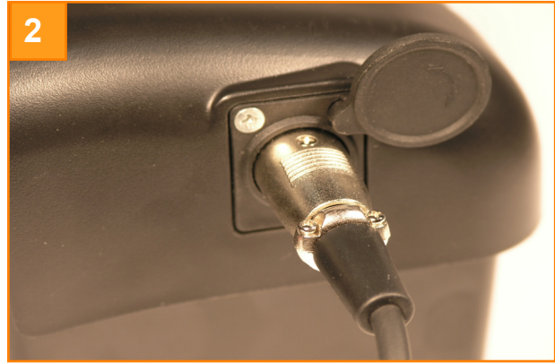
The charger output plug connects to the battery box.
