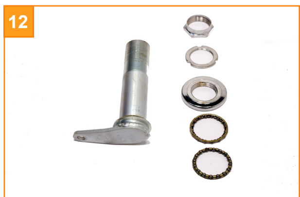
The steering stem showing the nut, locking ring, knurled ring & bearings.
