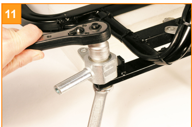
Use a 13.0 mm spanner/socket to undo the bolt securing the stub axle.
