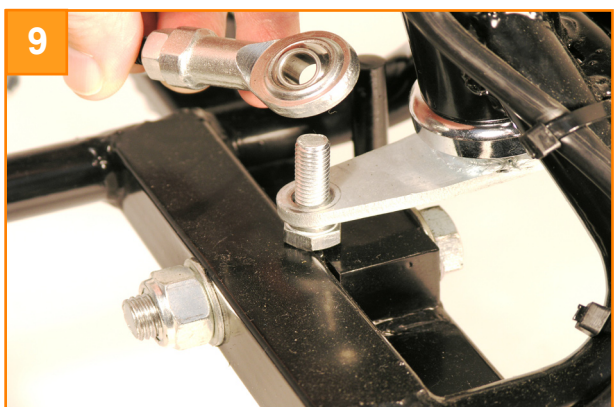
Lift the connecting rod off the bolt. Turn the steering to one side to remove the bolt.
