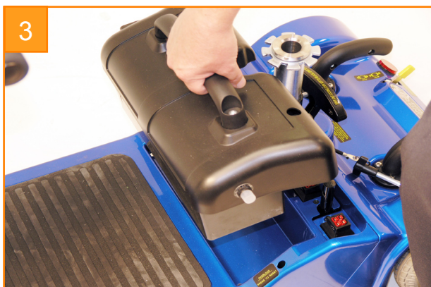
3 Lift the battery box off the scooter.
