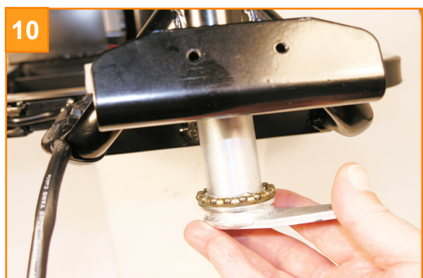
Slide the steering stem out of the head. The lower bearing should come with it, if not use thin nosed pliers to extract it from the head.
