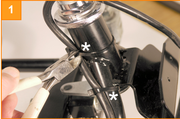
Cut the 2 cable ties on the steering head.
