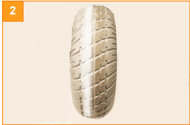
The tyre exhibits scuffing or a lightening of the tread colour on the outside half of the tyre. View from front of scooter.
