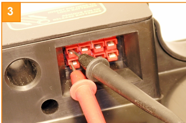
Place BLACK probe in top left & RED in bottom left sockets of the 8 pin plug . Do not short the probe pins.
