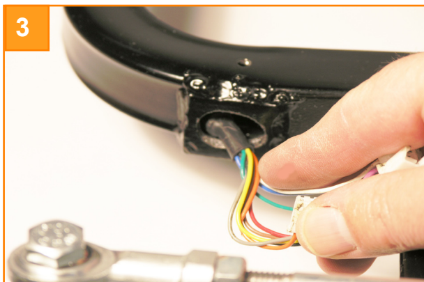
Feed the main loom into the hole at the front of the frame.
