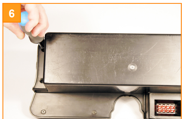
6 Use a Phillips screwdriver to undo the screws.
