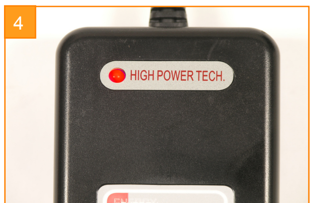
The top of the charger shows the charge status. RED LED = POWER ON
