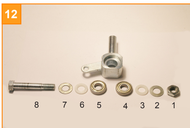
The stub axle removed showing the top to bottom sequence of nut, washers bearings & bolt.
