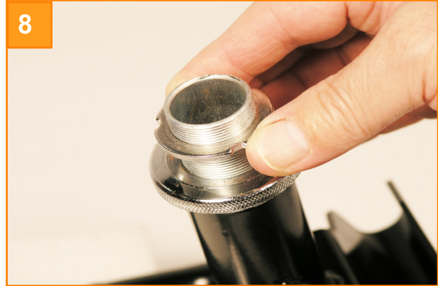
Remove the locking ring by hand.
