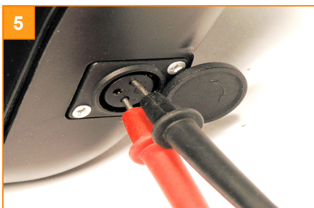
Place BLACK probe in pin 2 & RED in pin 1 as shown. Do not short the probe pins.
