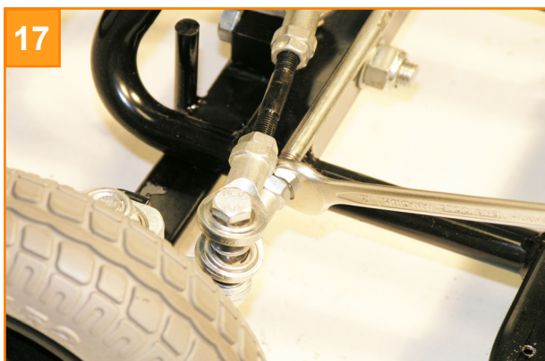
Carefully tighten the left hand nut using the 13.0 mm spanner.
