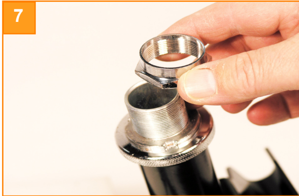
Remove the top nut by hand.
