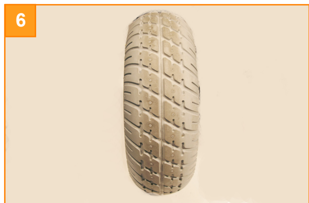
The tyre has no scuffing & any signs of normal wear are symmetrical.
