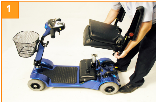
1 Push the seat lever forward & lift the seat off.
