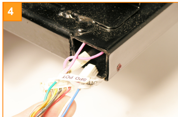
Simultaneously pull from the rear of the frame until the loom is through.
