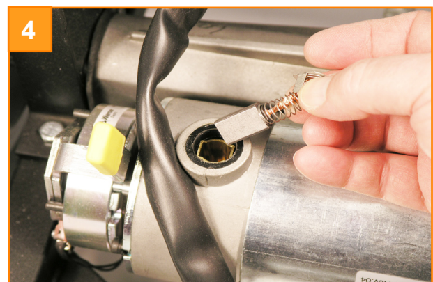
Gently pull the carbon brush out of the housing. Inspect the brush for cracks or chips. If the brush is a Blue colour, it may indicate excessive current. Check using a current clamp.
