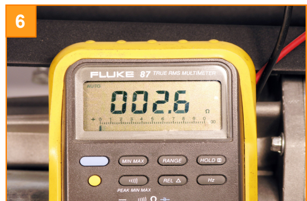
A low RESISTANCE reading should be displayed. If the reading is higher than 5.0 \Omega check the wiring for bad joints or signs of heat damage, if OK change the brushes. If still the same change the motor.
