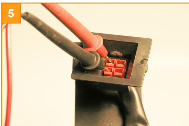
When the brushes are back in place insert the Multi-meter probes into the left hand pair of contacts (viewed from the rear).
