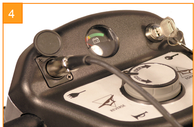
The charger output plug connects to the charging socket on the tiller top.
