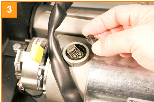
Carefully lift the brush cap off by hand. Do not loose the brush cap.
