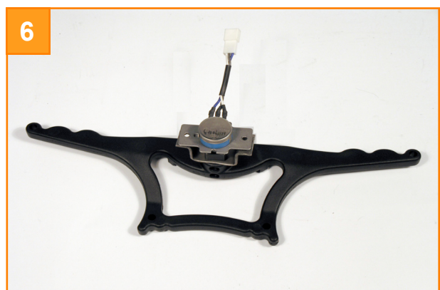
The wig wag throttle pot assembly removed, (shown inverted for clarity). Note that it is better to replace this part as a whole assembly, to preserve throttle calibration.
