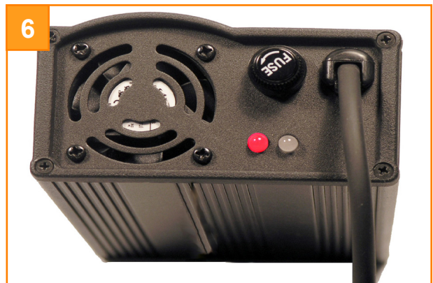
When there is mains power connected to the charger & the On/Off switch is turned ON, the RED LED illuminates.
