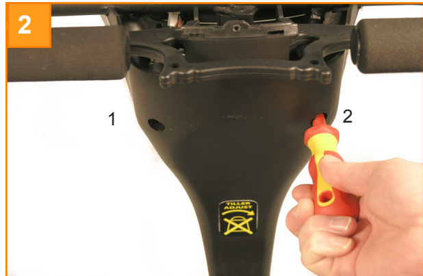
Use a Phillips screw driver to undo the 2 screws as shown above.
