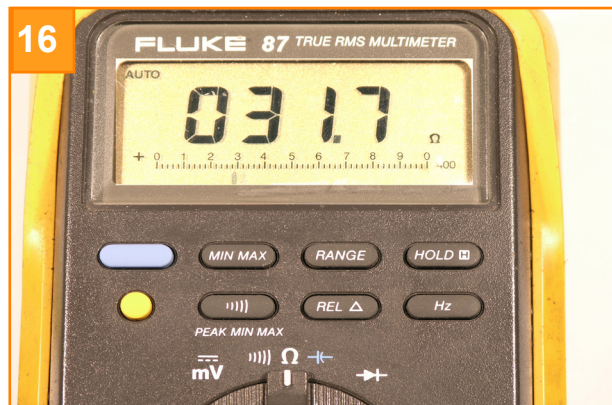
Set the meter to RESISTANCE. The meter should give an approximate reading between 25 - 35Ω.
