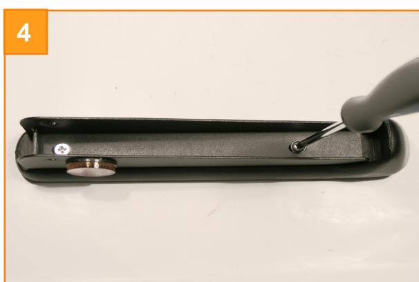
Invert the armrest & use a Phillips screw driver to undo the 2 screws. Note that the countersunk screw is towards the back.
