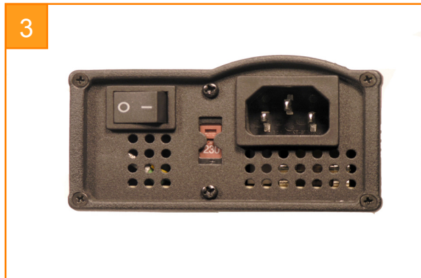
The rear panel has the On/Off switch, voltage change switch & power socket.
