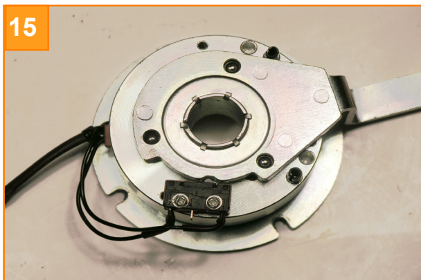
With the brake lever in the "DRIVE" position (micro-switch button out) insert the meter probes into the 2 pin plug.
