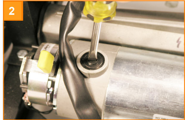
To access both of the motor brushes use a flat blade screw driver. One brush housing is on the top & one is underneath.
