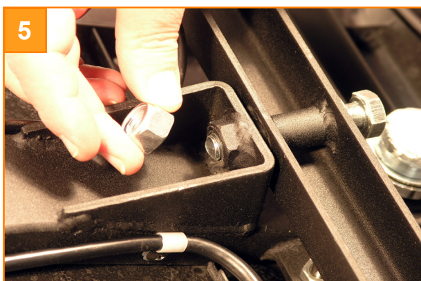
Remove the lock-nut & unscrew the bolt from the welded nut.
