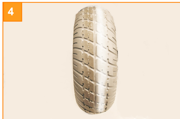
The tyre exhibits similar wear patterns as the tow in fault, but the damage is on the inside edge. View from front of scooter.
