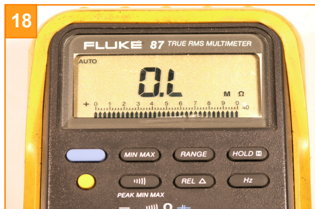
The meter should give an open circuit reading.
