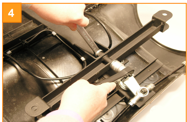
Use a 19.0mm spanner/socket to undo the lock nut on the front axle bolt.
